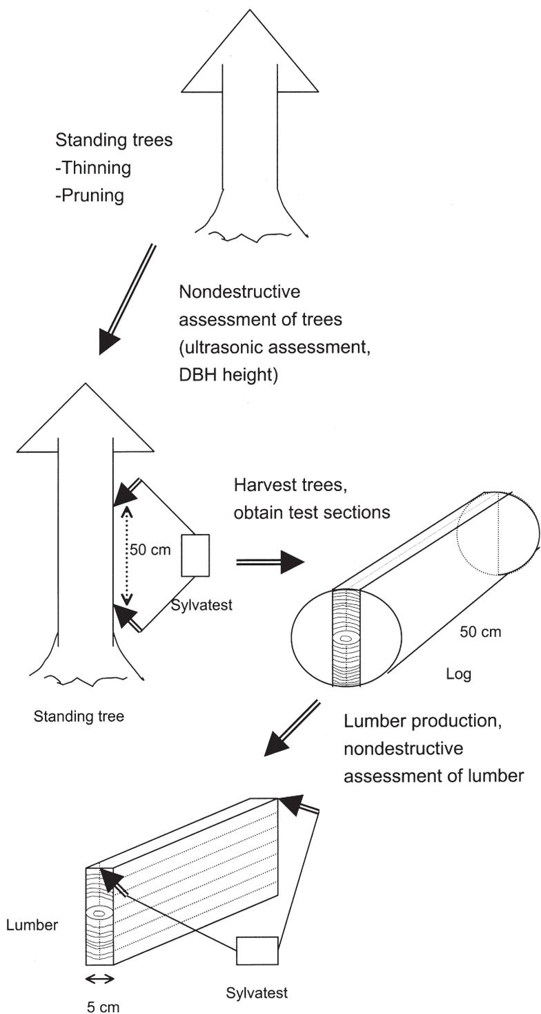
FIG. 1. Flow chart indicating the process of this study.
