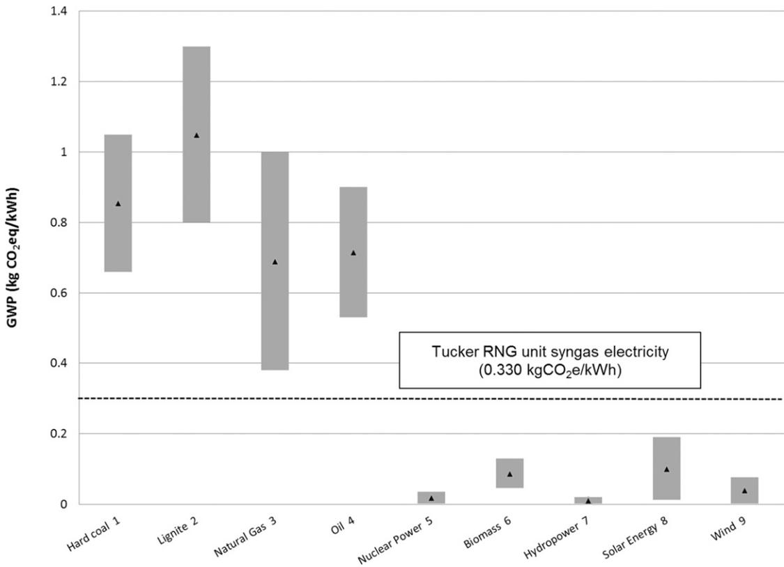
Figure 4. Global warming (GW) impact values for various electricity-generating technologies and the syngas electricity estimated in this study (RNG, renewable natural gas). Each bar represents the range of the GW values; midpoint on each bar represents the average represented GW.
