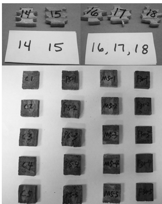
Figure 6. Block appearance for (top) southern pine controls and (bottom) untreated and treated pine scrim lumber after 28-da termite test (left to right: untreated controls, 5% phenolic formaldehyde [PF], 5% melamine formaldehyde [MF], 30% furfuryl alcohol [FA]).
