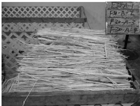
Figure 1. Typical scrim from the scrimming process (inset is the cross section of the panels).
