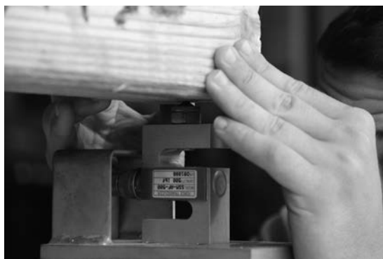
Figure 3. Transducer used for the E-computer test.
