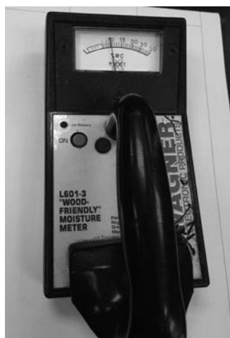
Figure 1. Wagner L601-3 handheld moisture meter.
