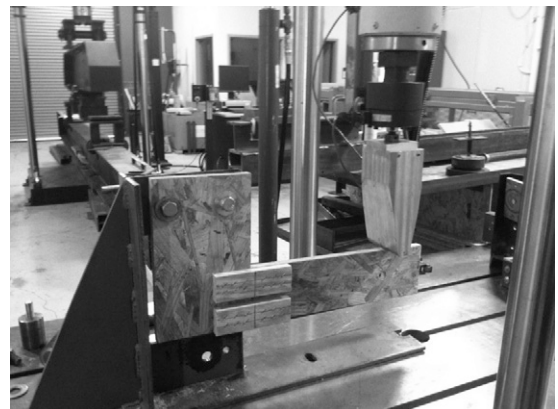
Figure 4. Test setup for the evaluation of in-plane bending moment resistance load capacity of T-shaped, one-sided, two-gusset-plate joints in oriented strandboard materials.
