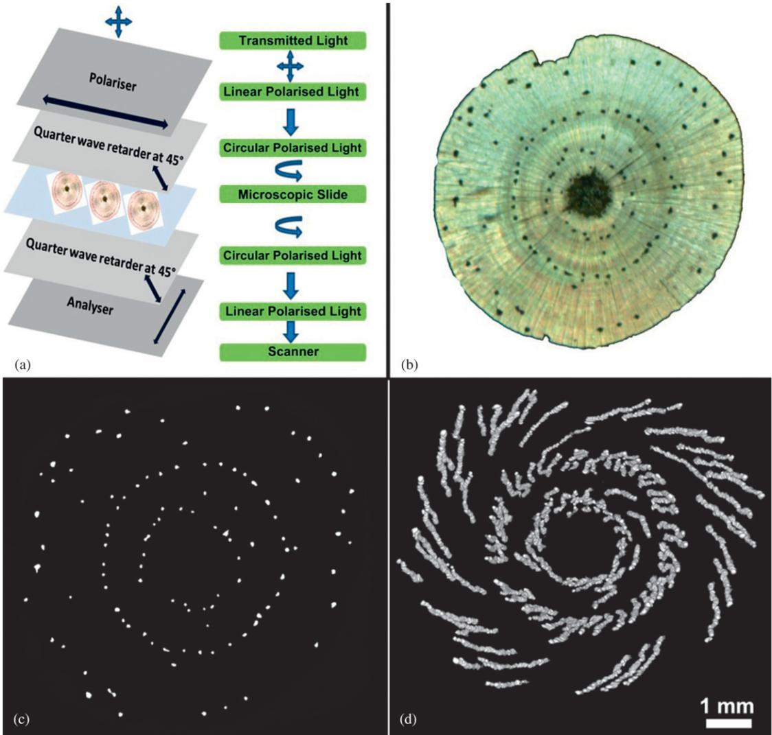
Figure 1. A new imaging and resin canal detection method reveals spiral grain. (a) Imaging with circular polarized light, (b) a transverse section imaged with circular polarized transmitted light, (c) resin canals (white dots) as detected with ImageJ, and (d) 3D visualization of resin canals and symmetric spiral grain in a vertical tree.
