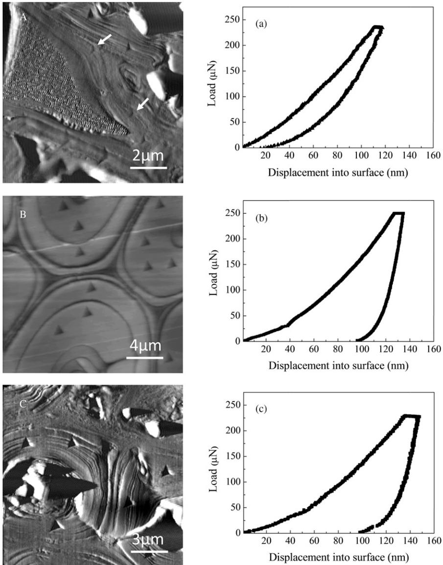
Figure 2. Residual indentations in the walls of different cell types ([A] silica cell, [B] bamboo fiber, [C] epidermal elongated cell) and the corresponding typical load-depth curves ([a] silica cell, [b] bamboo fiber [c] epidermal elongated cell).
