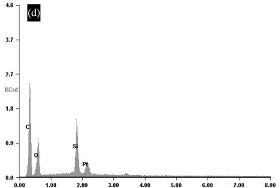
Figure 1. Cross section of (a) Moso bamboo, (b) its main cell type bamboo fibers, and (c) longitudinal sections of silica cells and epidermal elongated thick-walled cells located at the outermost layer of the bamboo. (d) Energy-dispersive X-ray analysis indicates the high silicon content of silica cells.
