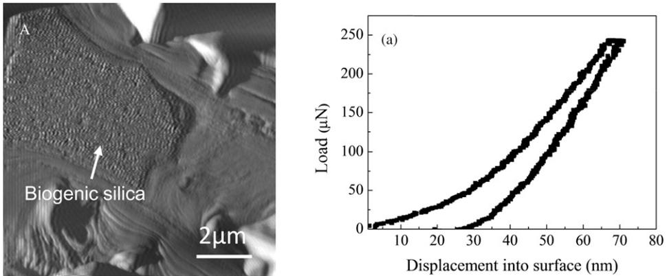
Figure 3. (A) Residual indentations in the pure biogenic silica and (a) the corresponding typical load-depth curves.
