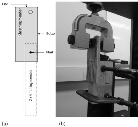
Figure 1. Connection geometry schematic (a) and test set-up (b).
