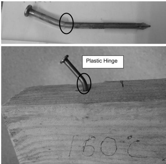
Figure 3. Two examples of mode III yielding.
