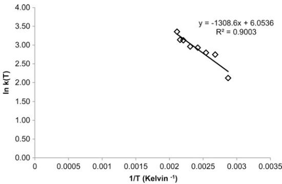
Figure 4. Natural log of  $k(T)$  as a function of  $1/T$  (absolute) demonstrating a good fit to Arrhenius activation energy theory.
