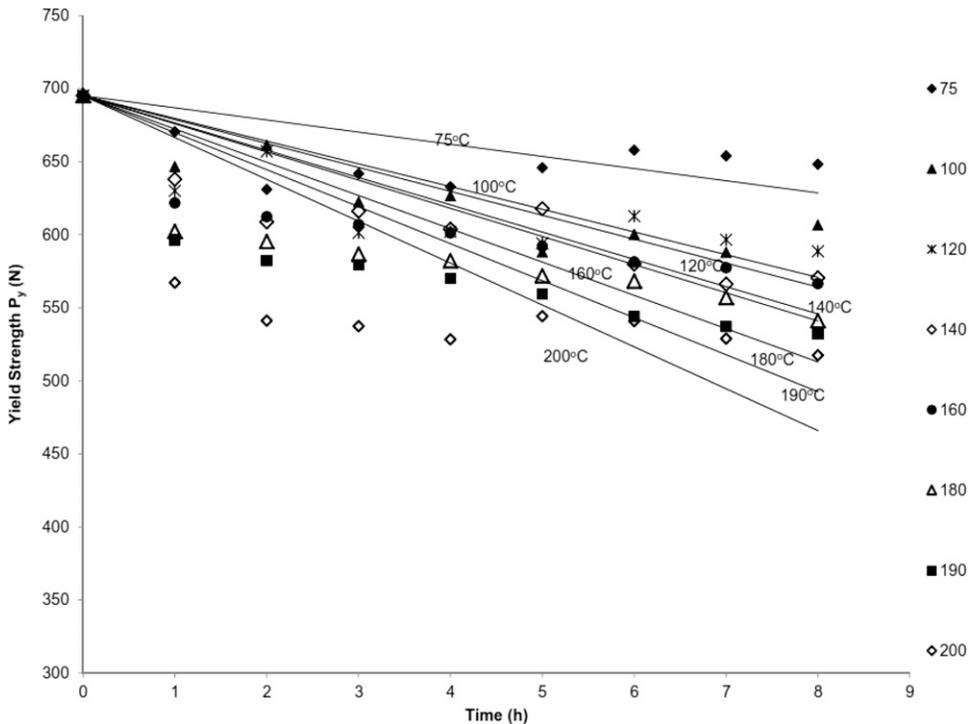
Figure 2. Yield strength of laterally loaded wood-to-OSB connections as a function of time and temperature.
