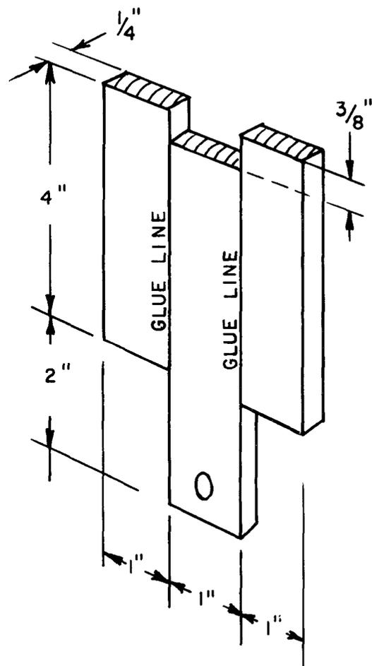
FIG. 2. Double shear specimen for shear modulus and creep measurement.
