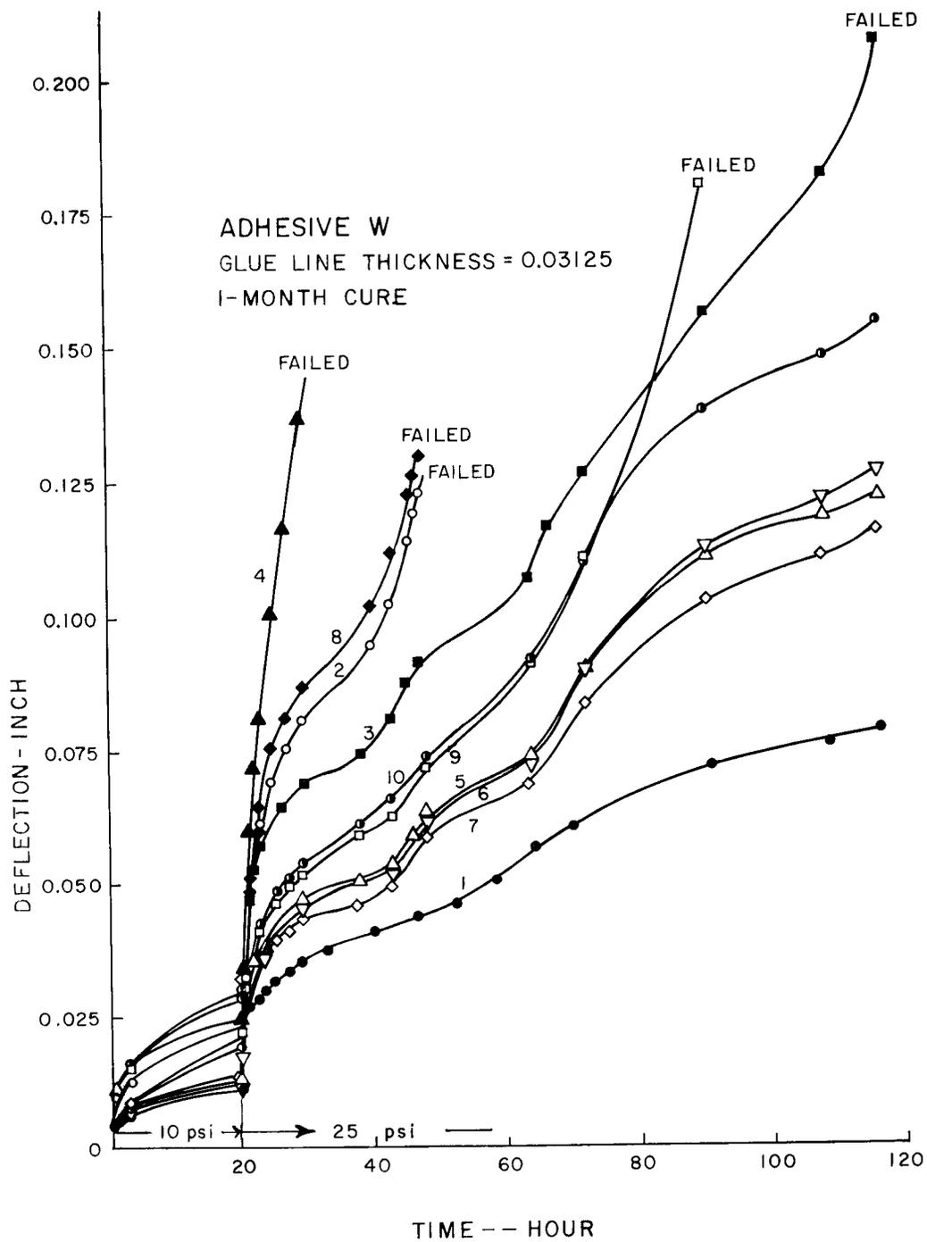
FIG. 7. Glue-line creep study of adhesive W, cured for 30 days.
