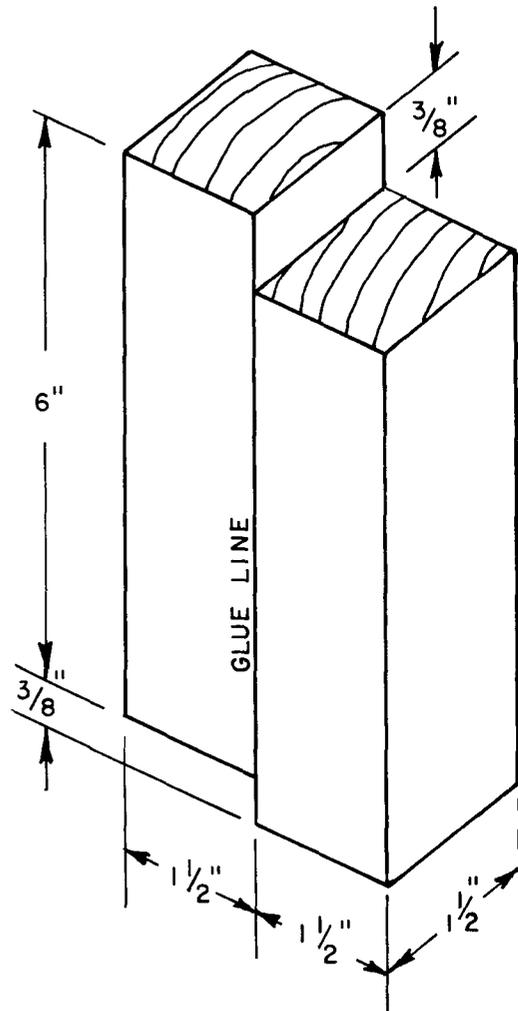
FIG. 1. Compression loaded block-shear specimen for shear strength testing.
