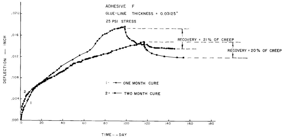
FIG. 6. Glue-line creep and recovery for adhesive F.
