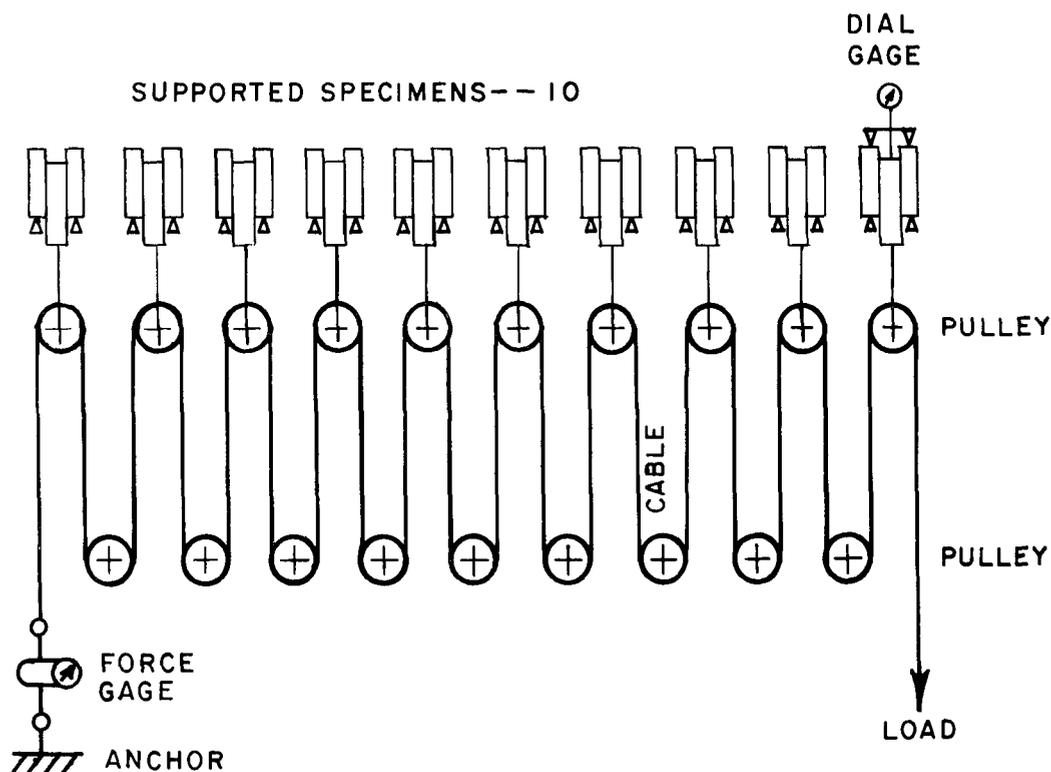
FIG. 3. Schematic diagram of test bench for measuring shear modulus, creep, and recovery.
