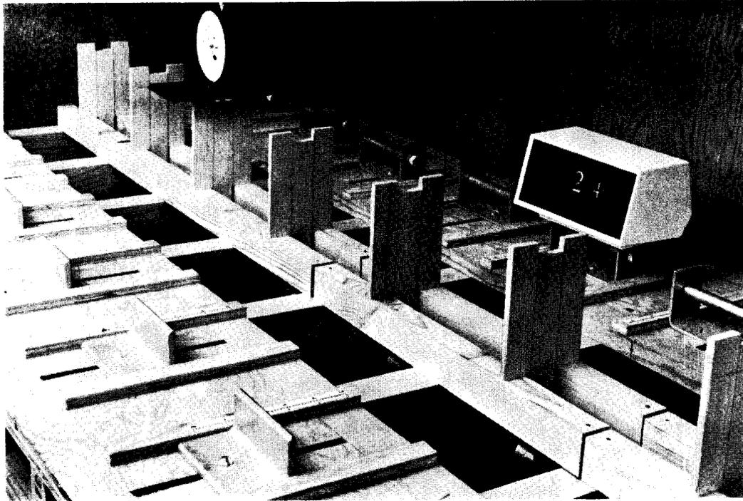
FIG. 4. Test bench for measuring shear modulus, creep, and recovery.
