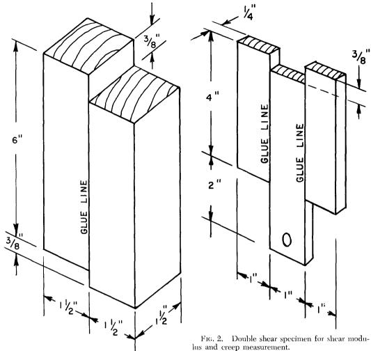
FIG. 1. Compression loaded block-shear specimen for shear strength testing.
