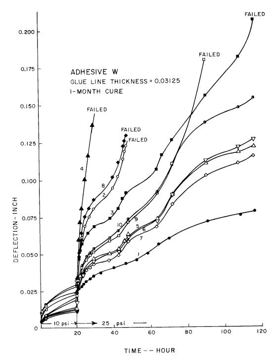
FIG. 7. Glue-line creep study of adhesive W, cured for 30 days.
