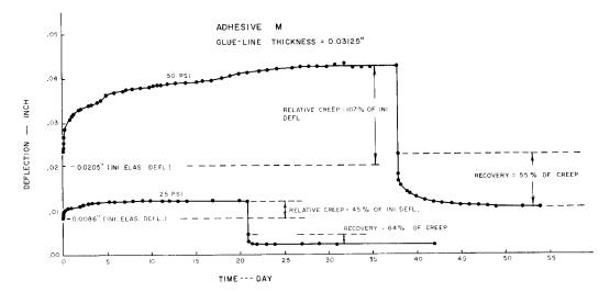
FIG. 5. Glue-line creep and recovery for adhesive M.
