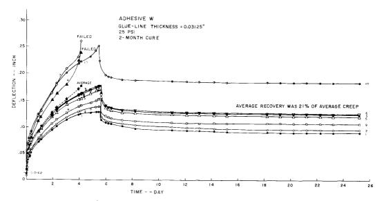
FIG. 8. Glue-line creep and recovery of adhesive W, cured for 60 days.
