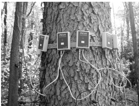
Figure 1. Acoustic tomography test on black cherry trees using a PiCUS ® Sonic Tomograph tool.
