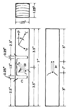
FIG. 1. Compression specimen for measuring shear modulus in the LT plane. Longitudinal direction L makes angle  $\alpha$  with load direction P. A, B, and C are strain gages mounted at 0°, 45°, and 90°, respectively, to the load axis. One-mil strain sensitive wires are shown as dashed lines. Solid connecting wires are 12 mils in diameter.
