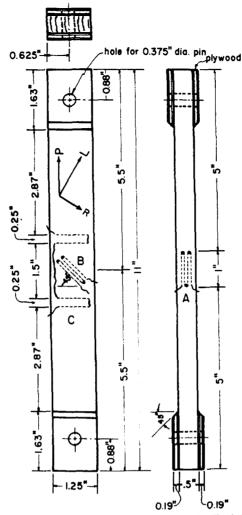
FIG. 2. Tension specimen for measuring shear modulus. Longitudinal direction L makes angle  $\alpha$  with load direction P. A, B, and C are strain gages mounted at 0°, 45°, and 90°, respectively, to the load axis. Shear modulus was in the LR plane for all tension specimens except sugar pine where measurements were in the LT plane. One-mil diameter strain sensitive wires are shown as dashed lines. Solid connecting wires are 12 mils in diameter.
