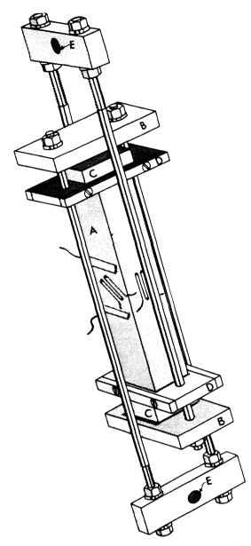
FIG. 3. Compression specimen A in compression cage. B is end block. C is end bearing block. D is centering guide. E is hole for metal dowel connection to universal joint. Ball bearing is centered between B and C at each end.
