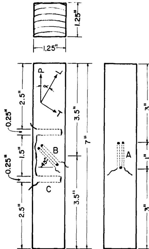
FIG. 1. Compression specimen for measuring shear modulus in the LT plane. Longitudinal direction L makes angle  $\alpha$  with load direction P. A, B, and C are strain gages mounted at  $0^\circ$ ,  $45^\circ$ , and  $90^\circ$ , respectively, to the load axis. One-mil strain sensitive wires are shown as dashed lines. Solid connecting wires are 12 mils in diameter.
