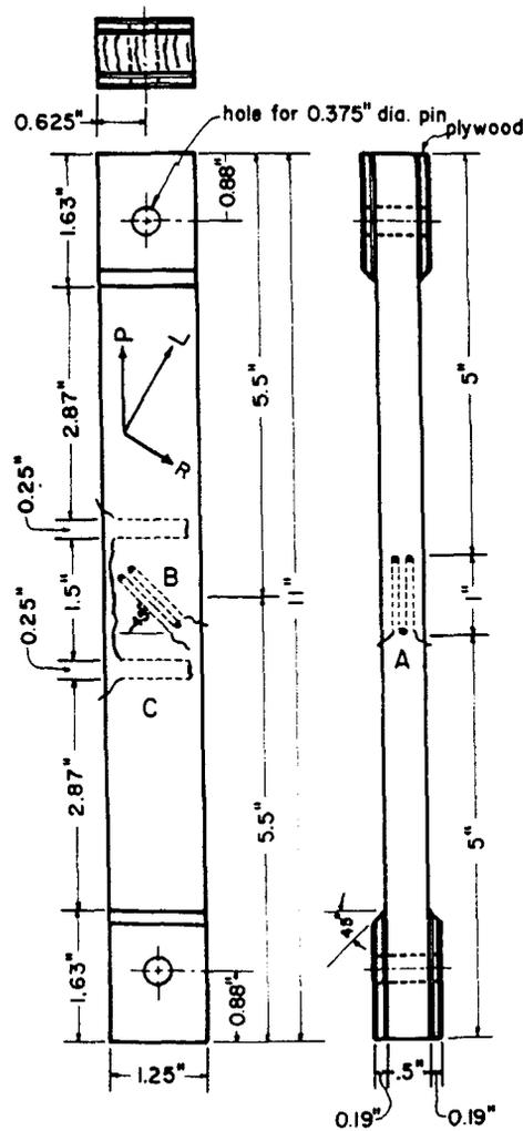
FIG. 2. Tension specimen for measuring shear modulus. Longitudinal direction L makes angle  $\alpha$  with load direction P. A, B, and C are strain gages mounted at  $0^\circ$ ,  $45^\circ$ , and  $90^\circ$ , respectively, to the load axis. Shear modulus was in the LR plane for all tension specimens except sugar pine where measurements were in the LT plane. One-mil diameter strain sensitive wires are shown as dashed lines. Solid connecting wires are 12 mils in diameter.
