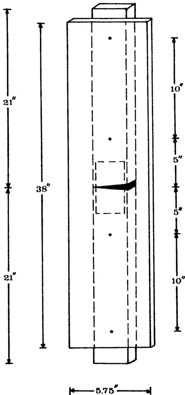
FIG. 3. Floor truss joint specimen. Gap is exaggerated for clarity.
