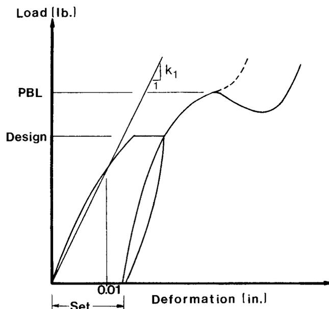
FIG. 4. Typical compression load-deformation curve for a splice joint. The solid line indicates the behavior of joints with  $\frac{1}{8}$  in. gap. The dotted line indicates post-buckling behavior of joints with  $\frac{1}{16}$  in. gap.
