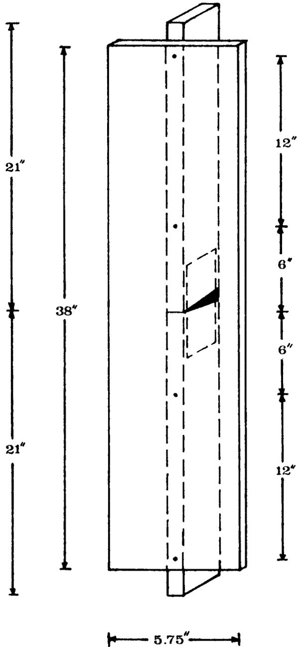
FIG. 2. Roof truss joint specimen. Gap is shown out of scale for clarity.
