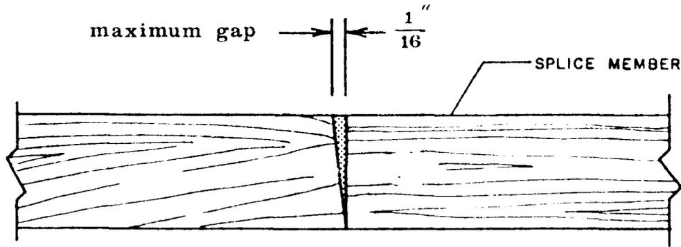
FIG. 1. Allowable manufacturing tolerance for compression splices per TPI QST-88.
