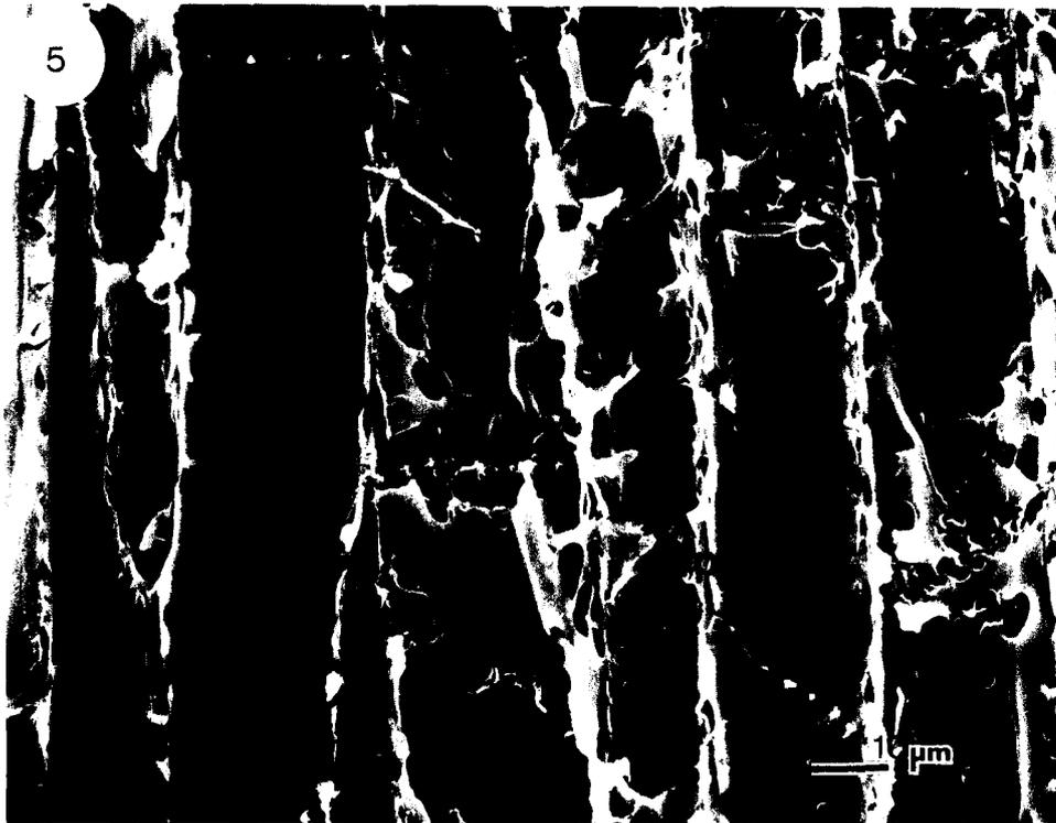
FIG. 5. Scanning electron micrograph of a smooth longitudinal split fracture plane along the growth ring boundary of wood decayed by *Bjerkandera adusta*. The lumen surface (Lu) was exposed during the fracture process indicating that failure was primarily transwall. Observe degradation of the ray parenchyma rp. Also notice hyphal sheath (hs) on the smooth fracture plane. cw is a marginal parenchyma cross wall.
