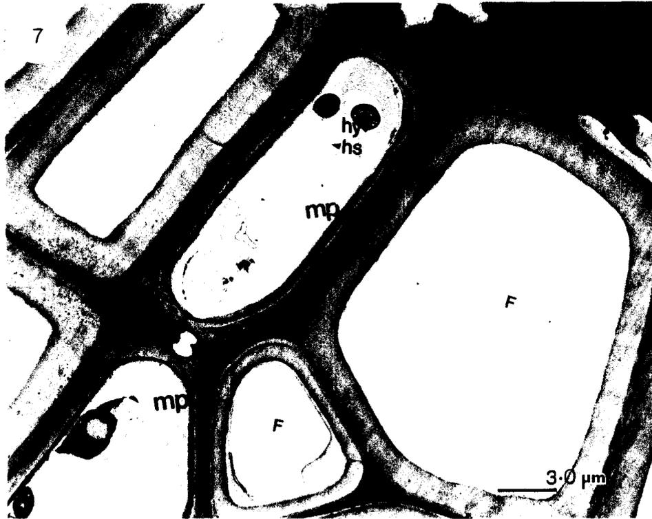
FIG. 7. Transmission electron micrograph of a cross-section of aspen decayed by *Bjerkandera adusta*. Notice fungal hyphae (hy) and hyphal sheath (hs) within lumen of the marginal parenchyma cells (mp). rp is the ray parenchyma region and F are fiber cells. The hyphae will only appear on the fracture plane when the lumen is opened (i.e., transwall failure).
