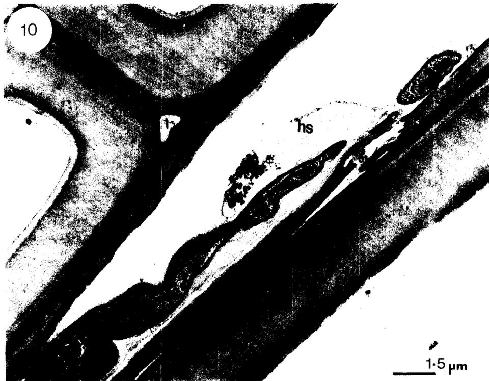
FIG. 10. Transmission electron micrograph showing invasion of a ray parenchyma cell by hypha (hy) and hyphal sheath (hs) of *Trametes versicolor*. I is an intercellular air space.
