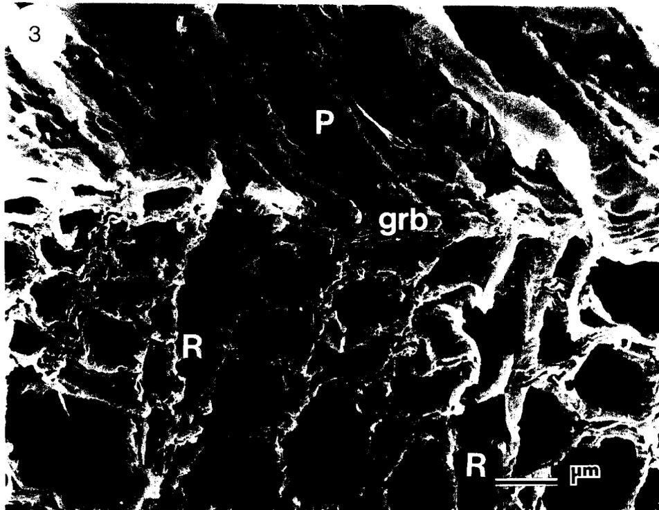
FIG. 3. Scanning electron micrograph of a smooth longitudinal split fracture plane (P) along the growth ring boundary of wood decayed by *Trametes versicolor*. Notice a gradual reduction in cell size from the bottom of the micrograph to the growth ring boundary. R indicates ray cells and tw indicates transwall failure.
