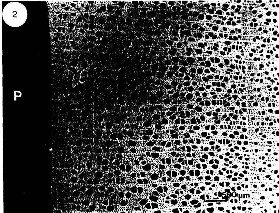
FIG. 2. Scanning electron micrograph showing that the fracture plane P associated with a longitudinal split failure (shown in Fig. 1a) was along the growth ring boundary (grb). The wood specimen examined here was decayed by *Trametes versicolor*.
