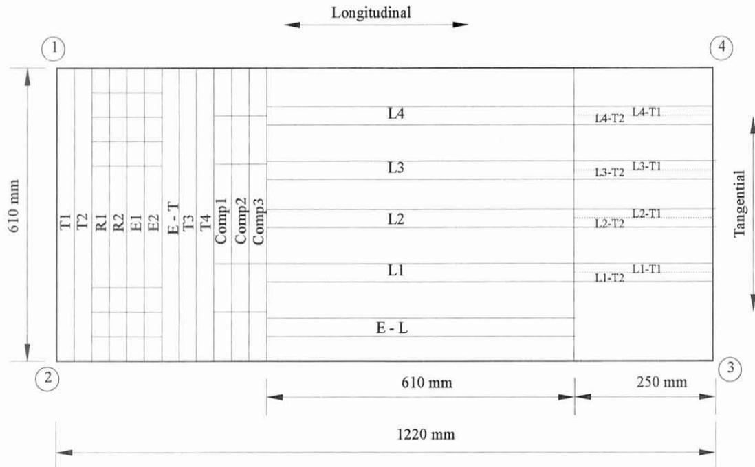
FIG. 4. Specimen arrangement on yellow-poplar test panel. E-L, E-T: longit. and tang. free hygroscopic expansion specimens; L1 . . . , T1 . . . : longit. and tang. beam laminas; L1T1 . . . : modulus of elasticity (tension) specimens; Compl . . . : modulus of elasticity (compression) specimens; R1 . . . : restraint test specimens; E1 . . . : free expansion specimens.
