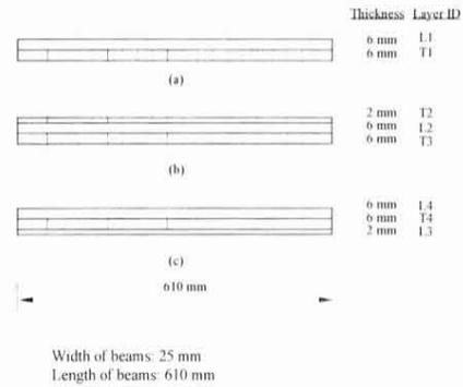
FIG. 5. Design of unbalanced yellow-poplar cross-laminated beams. Increase in relative humidity will cause beams to warp concavely upward. Note: L = longitudinal, T = tangential.
