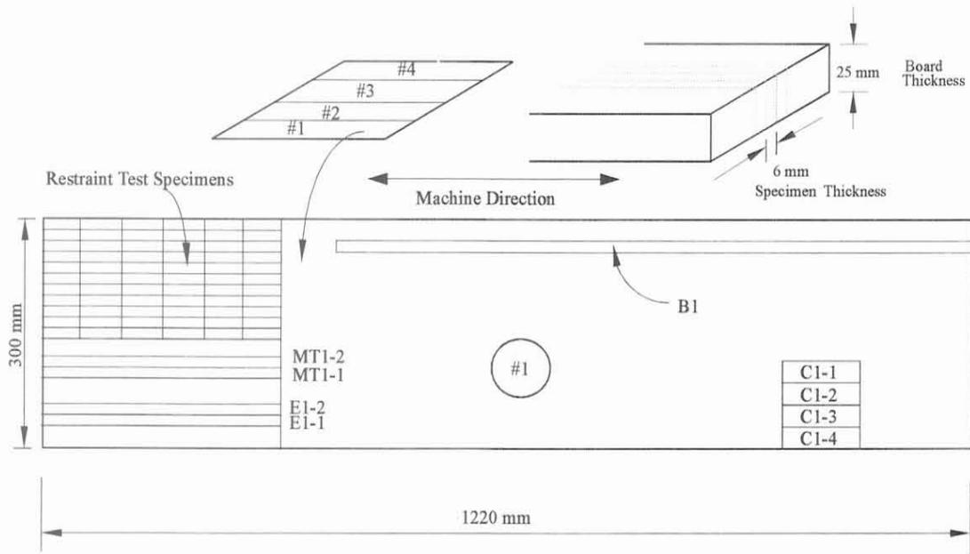
FIG. 6. Specimen arrangement on MDF and particleboard panels. Drawing shows one fourth of one panel. E1-1, E1-2: hygroscopic expansion specimens; B1: beam lamina; MT1-1, MT1-2: modulus of elasticity (tension) specimens; C1-1 . . . : modulus of elasticity (compression) specimens.
