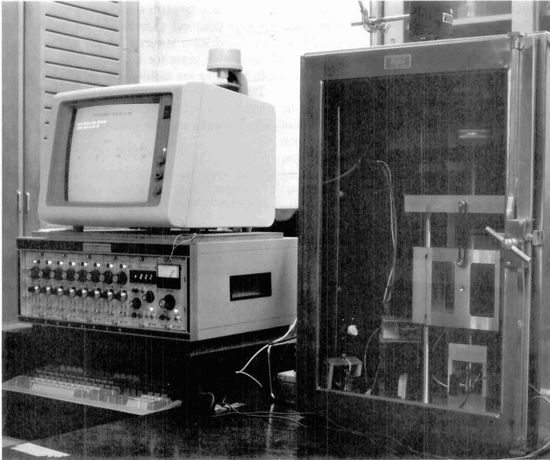
FIG. 10. Restraining device in climate chamber, and electronic data acquisition equipment.
