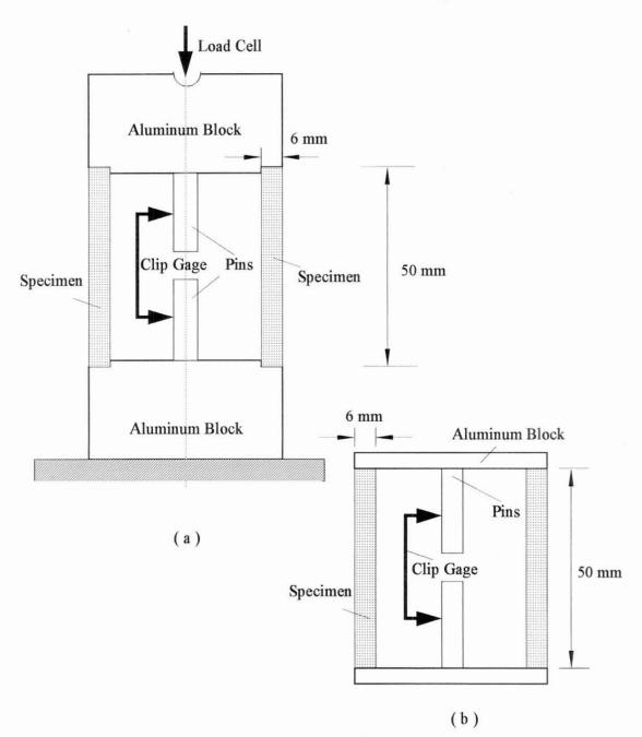
FIG. 8. Specimen placement in restraining device (a), and measurement of free hygroscopic expansion (b).
