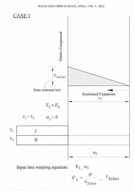
FIG. 1. Model of restrained swelling of laminas in two-layer unbalanced beam. Case I: complete restraint.
