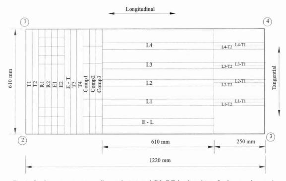
FIG. 4. Specimen arrangement on yellow-poplar test panel. E-L, E-T: longit. and tang. free hygroscopic expansion specimens; L1..., T1...; longit. and tang. beam laminas; L1T1...; modulus of elasticity (tension) specimens; Compl...; modulus of elasticity (compression) specimens; R1...; restraint test specimens; E1...; free expansion specimens.
