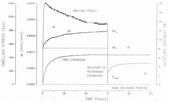
FIG. 9. Record of restrained swelling test of MDF. Specimens reached equilibrium at  $MC_2$  after about 70 hours. Upon removal of restraint, the instantaneous elastic recovery of the free expansion is determined. Swelling stress at that point is  $\sigma$ '.
