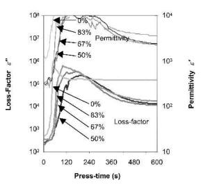
FIG. 6. Average phenol-formaldehyde dielectric loss-factor ( $\varepsilon''$ , log-scale) and permittivity ( $\varepsilon'$ , log-scale) signals from different thickness levels.
