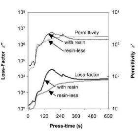
FIG. 8. Average resinless and phenol-formaldehyde dielectric loss-factor ( $\varepsilon''$ , log-scale) and permittivity ( $\varepsilon'$ , logscale) signals at the 50% thickness level for dry mats hotpressed at 2.4% moisture content.
