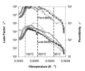
FIG. 7. Average phenol-formaldehyde resin loss-factor ( $\varepsilon''$ , log-scale) and permittivity ( $\varepsilon'$ , log-scale) versus the reciprocal of the average temperature measurements through the mat thickness. See Fig. 5 for legend.
