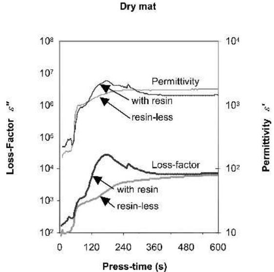
FIG. 8. Average resinless and phenol-formaldehyde dielectric loss-factor ( $\epsilon''$ , log-scale) and permittivity ( $\epsilon'$ , log-scale) signals at the 50% thickness level for dry mats hot-pressed at 2.4% moisture content.
