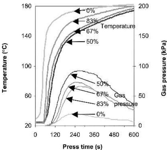
FIG. 4. Average internal temperature and gas pressure readings from different thickness levels.
