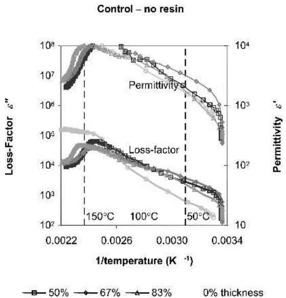
FIG. 5. Average loss-factor ( $\epsilon''$ , log-scale) and permittivity ( $\epsilon'$ , log-scale) versus the reciprocal of the average temperature measurements through the mat thickness with no exposure to phenol-formaldehyde resin.
