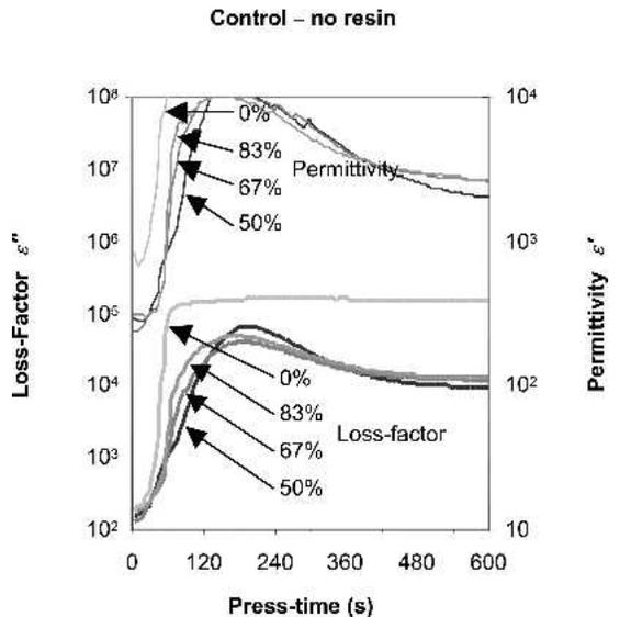
FIG. 3. Average control (no resin exposure) dielectric loss-factor ( $\epsilon''$ , log-scale) and permittivity ( $\epsilon'$ , log-scale) signals from different thickness levels (0% to 83% thickness).
