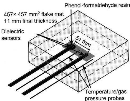
FIG. 2. Experiment setup. Two implanted dielectric analysis sensors (one exposed to a layer of phenol-formaldehyde resin), and two implanted temperature/gas pressure probes.
