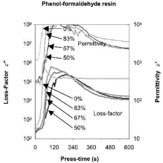
FIG. 6. Average phenol-formaldehyde dielectric loss-factor ( $\epsilon''$ , log-scale) and permittivity ( $\epsilon'$ , log-scale) signals from different thickness levels.
