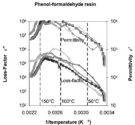
FIG. 7. Average phenol-formaldehyde resin loss-factor ( $\epsilon''$ , log-scale) and permittivity ( $\epsilon'$ , log-scale) versus the reciprocal of the average temperature measurements through the mat thickness. See Fig. 5 for legend.
