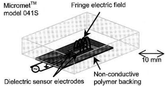
FIG. 1. Fringe-field dielectric ribbon sensor schematic. Fringe electric field through the mat, from a low voltage alternating current.
