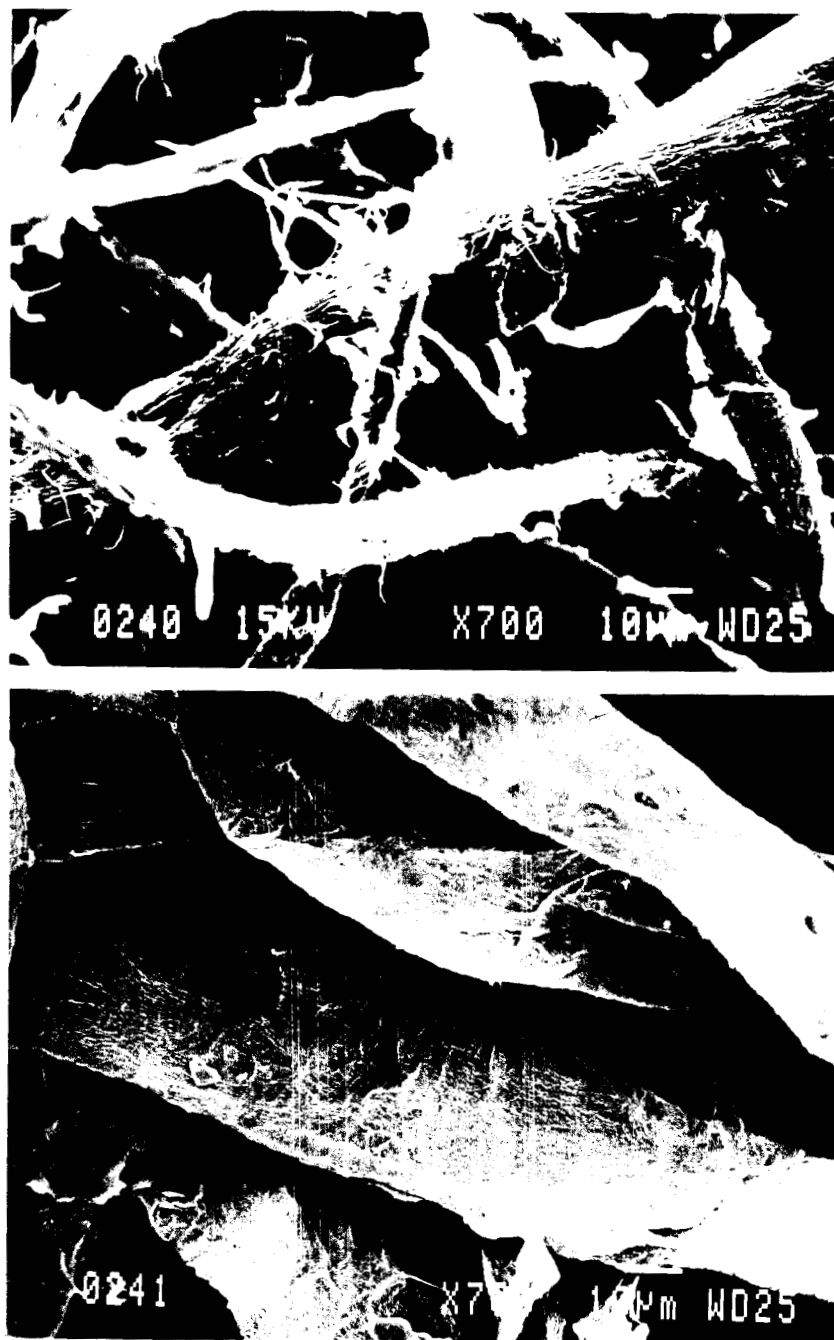
FIG. 4. SEM micrographs of recycled fiber from linerboard. Top: Hexamethyldisilazane-treated, 590 CSF, 700 \times ; Bottom: nontreated, 495 CSF, 700 \times . (MC87 9010)
