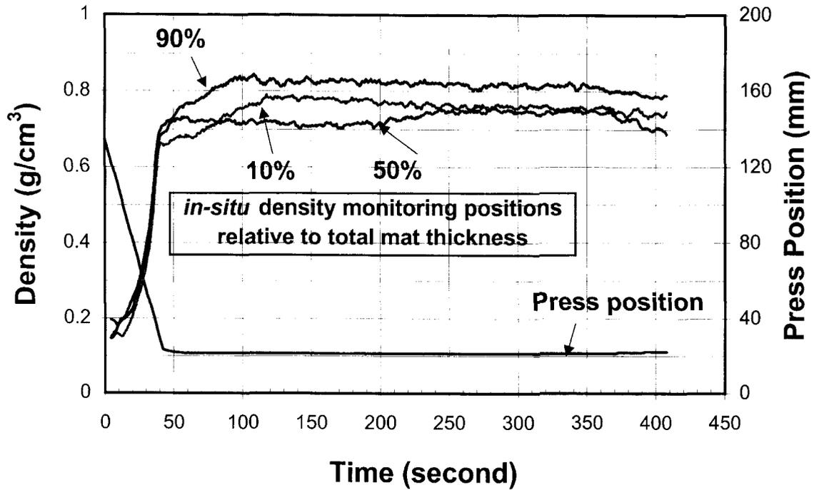
FIG. 3. In-press densities of a pine OSB mat pressed at a 40-s closure rate.
