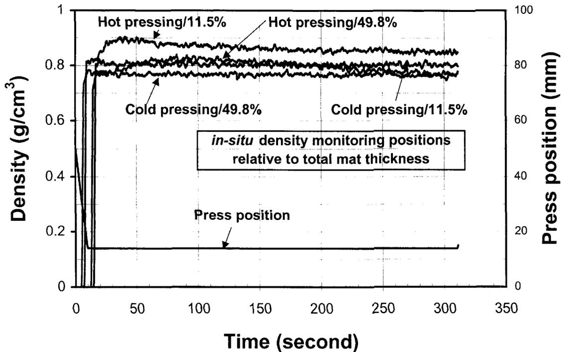
FIG. 5. A comparison of density changes in 12.7-mm thick MDF panel when pressed hot and when pressed cold.
