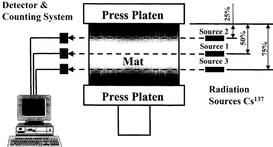
FIG. 2. A schematic representation of the *in-situ* density monitoring system.
