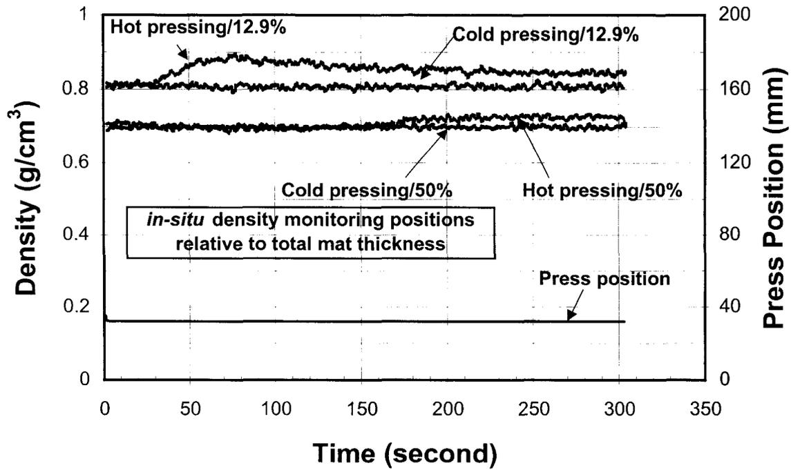
FIG. 4. A comparison of density changes in a 25.4-mm-thick MDF panel when pressed hot and when pressed cold.
