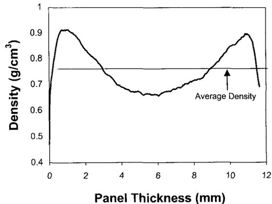
FIG. 1. Typical density profile shape that is nearly symmetrical through the board thickness.
