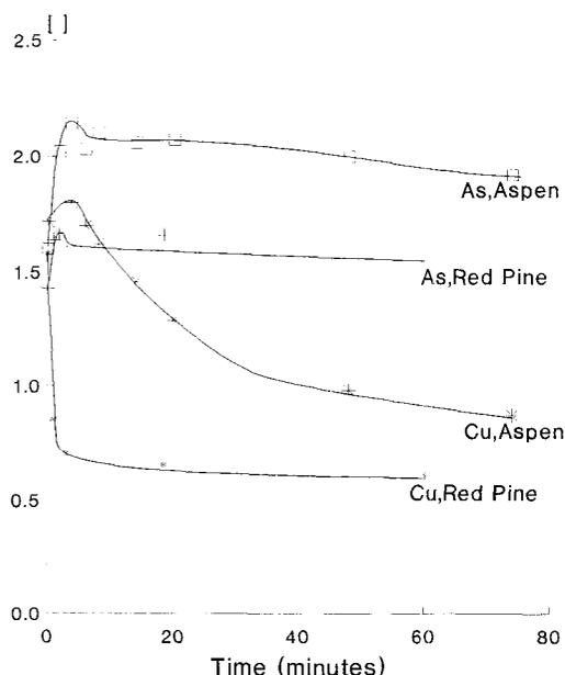
FIG. 6. Change in concentration of copper and arsenic in solution expressed from wood void space following treatment with ammoniacal copper arsenate.
