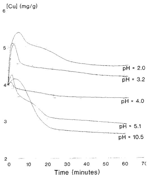
FIG. 3. Change in concentration of copper in solution expressed from wood void space as affected by solution pH—aspens at low moisture content.
