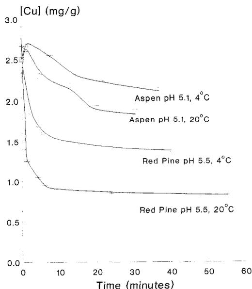
FIG. 2. Change in concentration of copper in solution expressed from wood void space as affected by species and ambient temperature.
