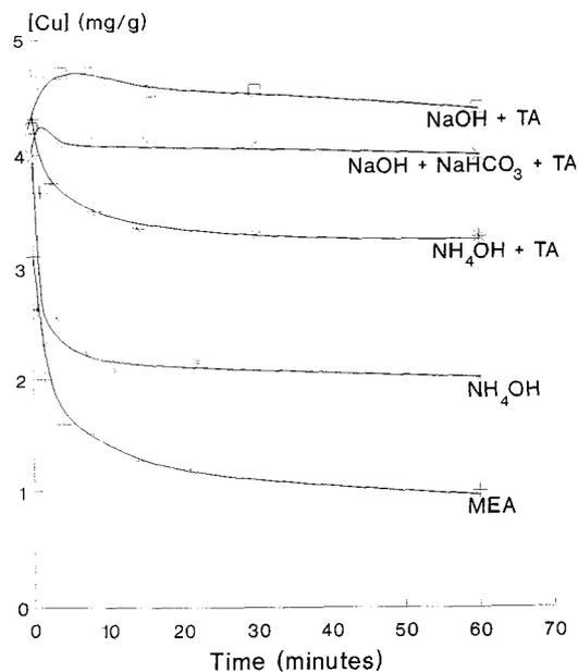
FIG. 4. Change in concentration of copper in solution expressed from wood void space from various high pH systems—red pine at initial pH = 10.5.
