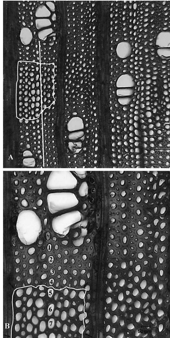
FIG. 3. Micrographs of tension wood of sugar maple stained with safranin and astra blue in aqueous solution. A shows a row of cells (white line) formed by the “same” initial. B shows an enlarged part of A pointing out part of the libriform fiber region (encircled area with arrows). Observe the difference in cell diameter and the differences in staining reaction (darker) in the libriform fiber regions (encircled area of B). Cells 1-4 are fiber tracheids; cells 5 to 7 are libriform fibers.
