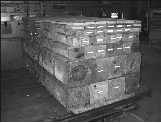
FIG. 1. Stack of ponderosa pine boards and square timbers ready for the kiln. This figure shows stickers between layers of boards/squares, but the data for this study were taken from unstickered stacks. Pieces with white tags have thermocouples embedded in their center.
