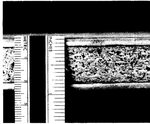
FIG. 2. Sandwich floor system consisting of \frac{5}{8} -inch particleboard core reinforced on each face with \frac{1}{8} -inch southern pine veneer.
