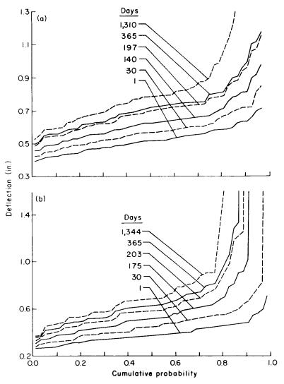
FIG. 11. Cumulative frequencies of total deflections of SS and No. 2 specimens at selected times during the first 3.5 years under sustained constant load in an uncontrolled environment: (a) 50 SS specimens, (b) 50 No. 2 specimens. (ML90 5375)
