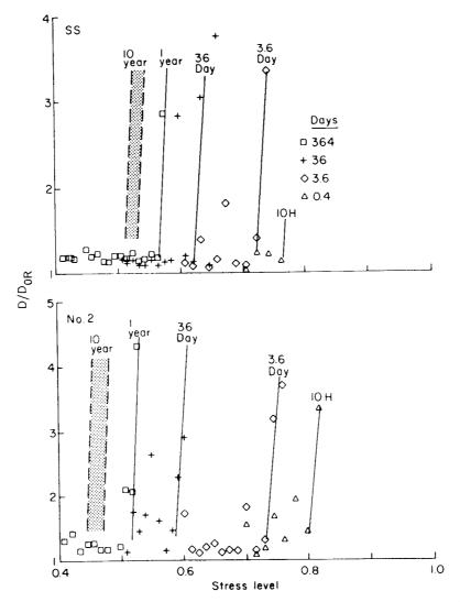
FIG. 9.  $D/D_{0R}$  relative to SL and time overlaid with maximum predicted trend lines. (ML90 5373)
