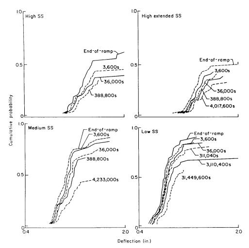
FIG. 6. Cumulative distributions of SS specimen deflections at selected times in seconds after start of ramp loading. End-of-ramp loading is  $T_0$  in Table 3. (ML90 5382)
