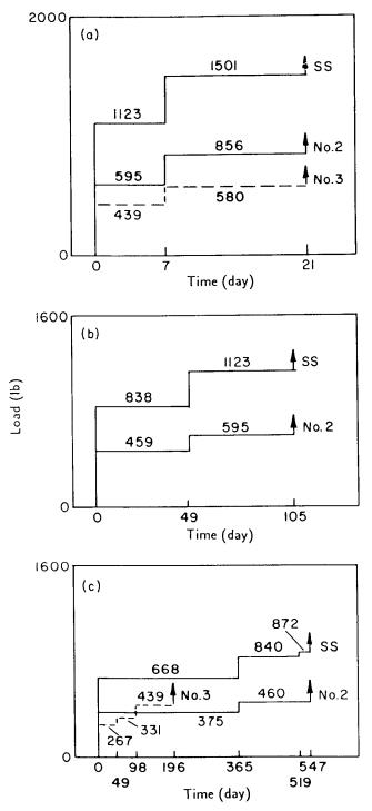
FIG. 2. Experimental load durations at 73°F, 50% relative humidity: (a) High step-constant-load series, (b) medium step-constant-load series, (c) low step-constant-load series. Change in step-constant-load levels within a series at 300 lb/min. One pound of load equals 5.13 lb/in.<sup>2</sup> bending stress. (ML90 5368)
