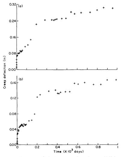
FIG. 10. Examples of creep deflection in an uncontrolled environment. (a) SS  $D_0 = 0.484$  in., (b) No. 2  $D_0 = 0.357$  in. (ML90 5374)
