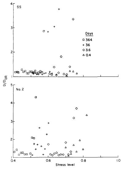
FIG. 8.  $D/D_{0R}$  relative to SL and time for low step-constant-load specimens. Excludes specimens with SL <0.4 for 364 days, <0.5 for 36 days, <0.6 for 3.6 days , and <0.7 for 10 h. (ML90 5372)
