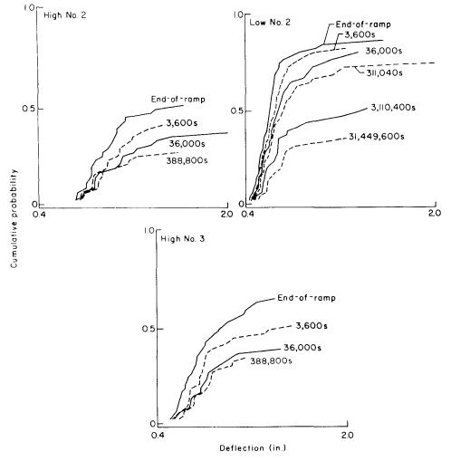
FIG. 7. Cumulative distributions of No. 2 and No. 3 specimen deflections at selected times in seconds after start of ramp loading. End-of-ramp loading is  $T_0$  in Tables 4 and 5. (ML90 5381)
