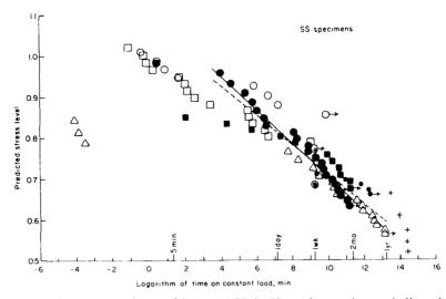
FIG. 14. Relation between time to failure and SL in SS specimens. Arrows indicate incomplete tests. Solid line indicates regression; broken line indicates alternate regression with SL as dependent variable. Data point +, 412.7 lb (uncontrolled environment). Other data points from Gerhards (1988, controlled environment). (ML90 5379)
