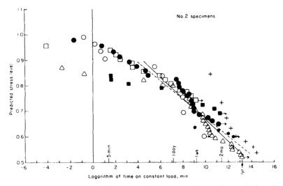
FIG. 15. Relation between time to failure and SL in No. 2 specimens. Arrows indicate incomplete tests. Solid line indicates regression; broken line indicates alternate regression with SL as dependent variable. Data point +, 232 lb (uncontrolled environment). Other data points from Gerhards (1988, controlled environment). (ML90 5380)
