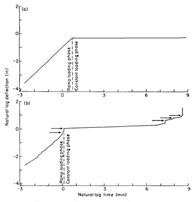
FIG. 3. Examples of log-log plots of total deflection as a function of total time at test. (a) SS specimen without failure during first step of low step-constant-load test (668 lb). (b) No. 2 specimen of low step-constant-load test (375 lb) with several partial failures (arrows) before complete failure. (ML 90 5369)
