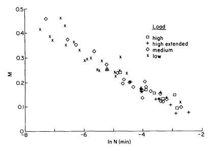
FIG. 4. Correlation of creep parameters, M and ln N, for 64 SS specimens. (ML90 5370)
