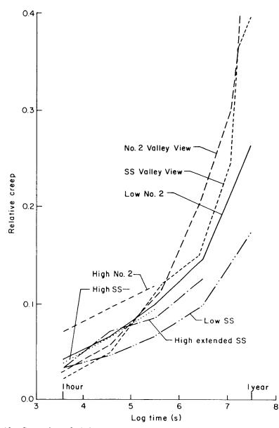
FIG. 13. Comparison of relative creep at 20th percentile of sample populations in controlled and uncontrolled environments. No. 2 and SS Valley View are for uncontrolled environment, others for controlled environment. (ML90 5378)
