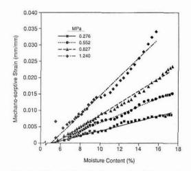
FIG. 4. The relationship between mechano-sorptive strain and moisture-content change at different stress levels. Lines show the linear fits.
