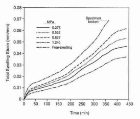
FIG. 3. Total swelling strain as a function of time at four stress levels. The curve for free-swelling samples is the mean for the four tests. Load was applied at time zero.
