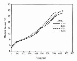
FIG. 2. Moisture-content change as a function of sorption time at four stress levels.
