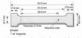
FIG. 1. Test specimen with reference mark for strain measurement.
