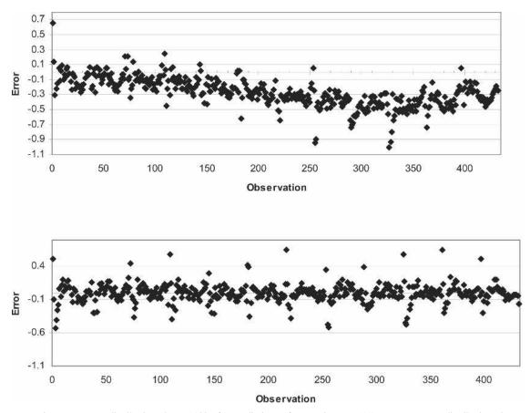
FIG. 3. Top: Error distribution above 110°F for predictions of regression Eq. (11); Bottom: Error distribution above 110°F for predictions of regression Eq. (12).
