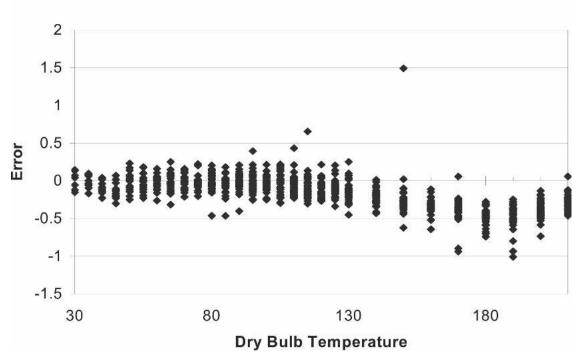
Error in EMC prediction vs Dry Bulb Temperature
