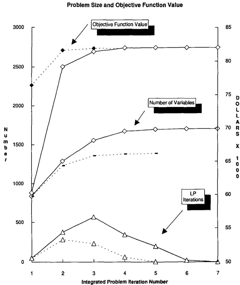
FIG. 5. A comparison of the efficiency of solving the sample problem between using final shadow prices (dashed lines) and demand group 1 prices (solid lines) as first iteration inputs.
