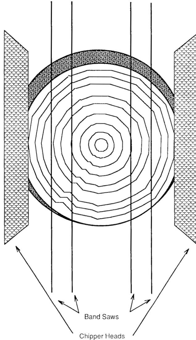
FIG. 1. Placement of saws and chipper heads in the chipper-canter QUAD bandmill.
