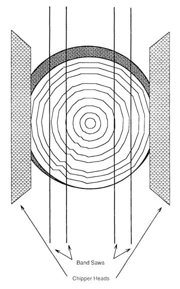
FIG. 1. Placement of saws and chipper heads in the chipper-canter QUAD bandmill.
