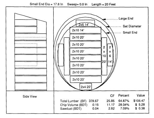
FIG. 2. A sawing pattern for the QUAD bandmill developed by the cutting pattern optimizer.
