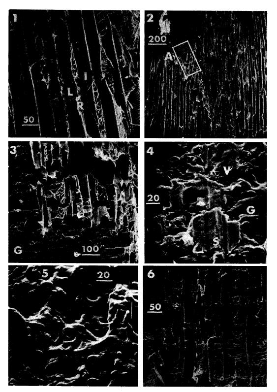
ular to the tracheid axis is the least common type of failure.
