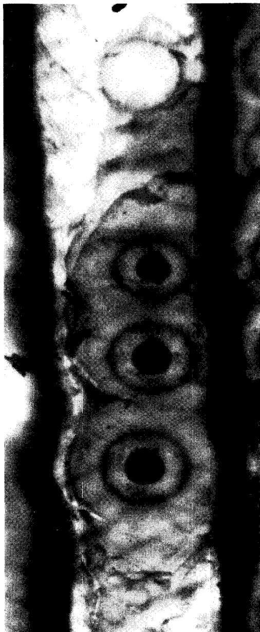
FIG. 2. Radial section of Douglas-fir showing some fracturing of layers of the tracheid wall during cutting in the direction of the fiber axis; 6 \mu m, Karo mount.
