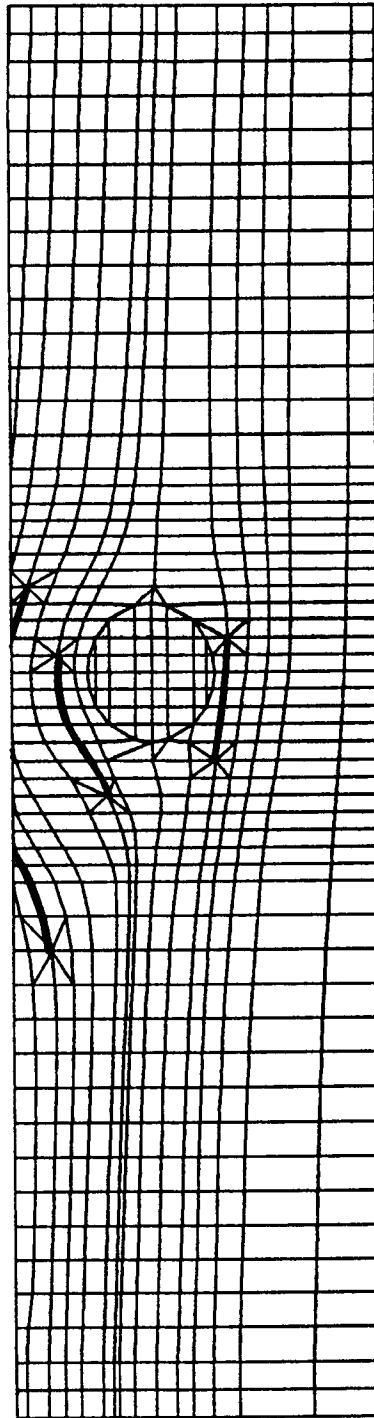
FIG. 8. Typical finite element mesh displaying accumulated fractures as indicated by the bold lines surrounded at each crack tip by eight triangular singular elements.
