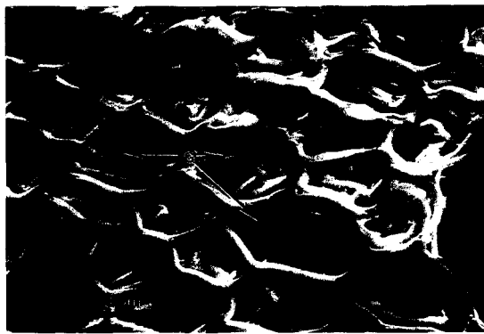
FIG. 3. Specimen 2b with thick-walled gelatinous fibers (G) from the center of the same growth increment shown on the right side of Fig. 2 ( \times 1,250 ).
