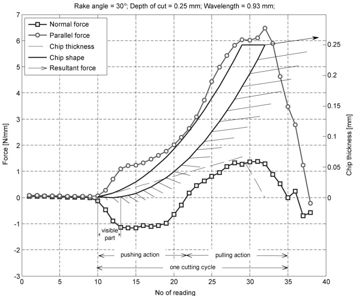
Figure 2. Progression of parallel and normal cutting forces during an individual chip length along with the theoretical chip shape and chip thickness. Resultant force is also represented by successive vectors.
