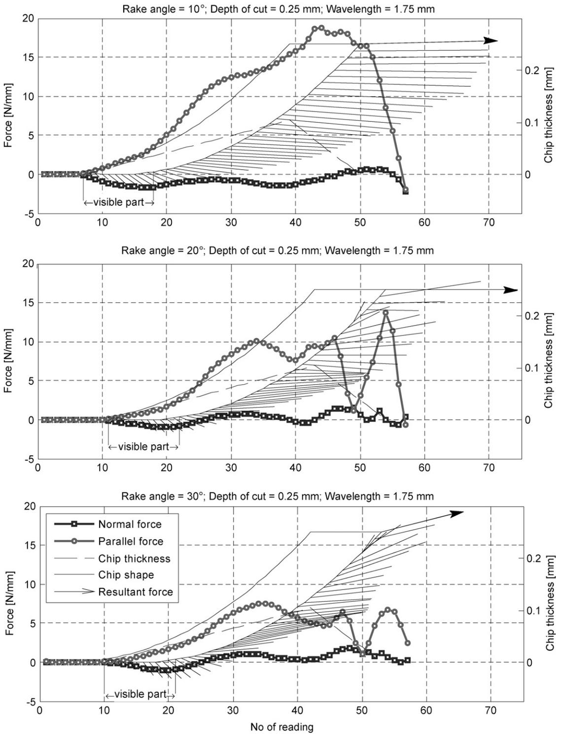
Figure 4. Effect of rake angle on cutting forces.
