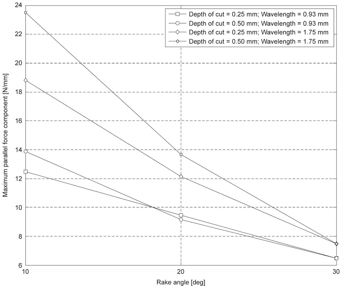
Figure 3. Maximum parallel force component as a function of rake angle, depth of cut, and wavelength.
