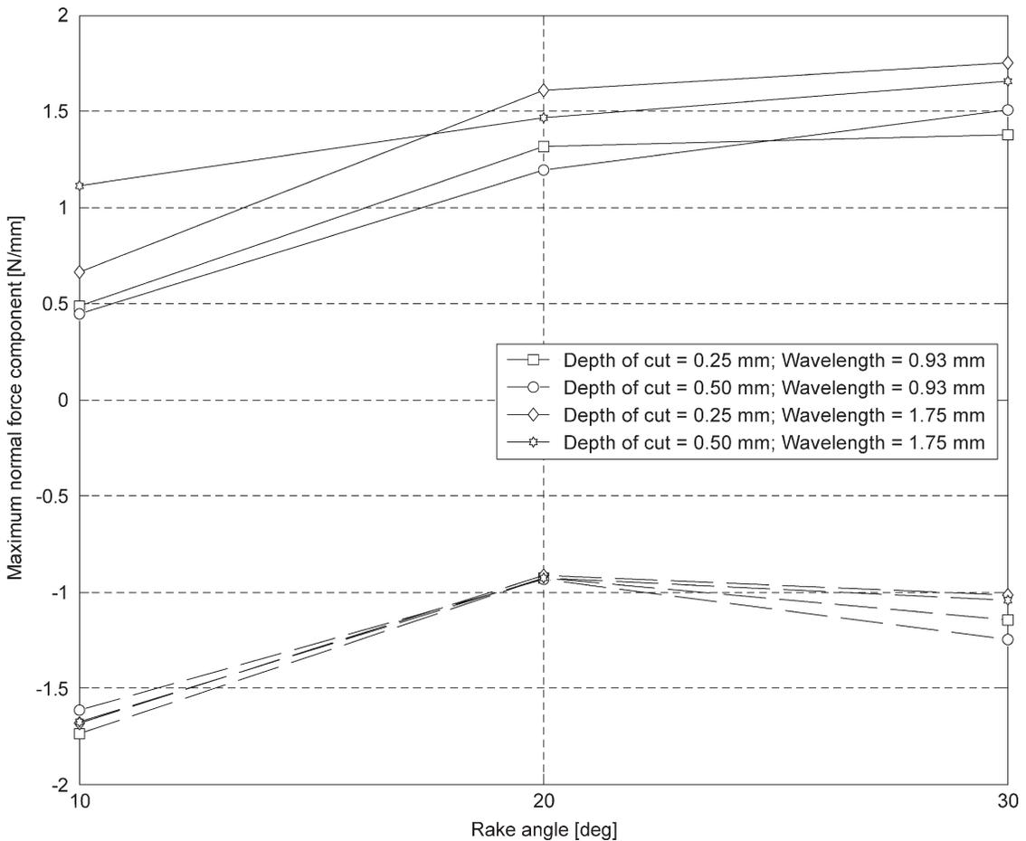
Figure 5. Maximum normal forces for both negative (pushing) and positive (pulling) components as a function of rake angle, depth of cut, and wavelength.
