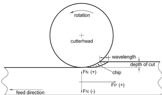
Figure 1. Parallel  $F_P$  and normal force  $F_N$  components during up-milling. Diagram shows that  $F_N$  can act upward (positive value) or downward (negative value).
