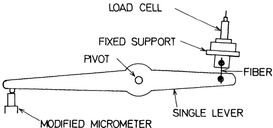
FIG. 2. Fiber microtensometer used to fracture small specimens.
