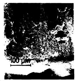
FIG. 4. Cross-section of large specimens showing (1) bundles of narrow lumen fibers, (2) very large xylem vessels, and (3) broad lumen parenchyma cells.
