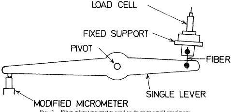
FIG. 2. Fiber microtensometer used to fracture small specimens.
