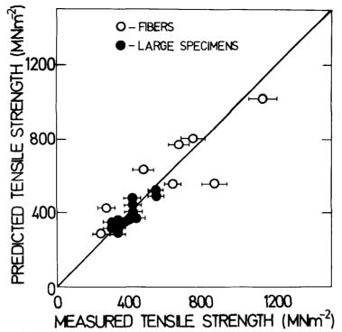
FIG. 3. Evaluation of empirical equations for the tissue of small specimens (labelled as fibers) and large specimens.
