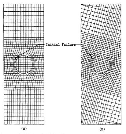
FIG. 2. Program STARWX predicted initial failure to occur due to shear stress at the location indicated.
