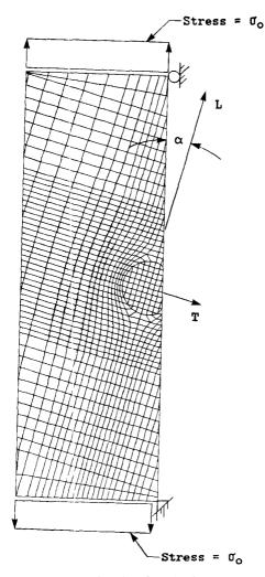
FIG. 1. Finite element mesh approximation for edge-knot member with global grain angle  $\alpha$ , generated by Program STARWX.
