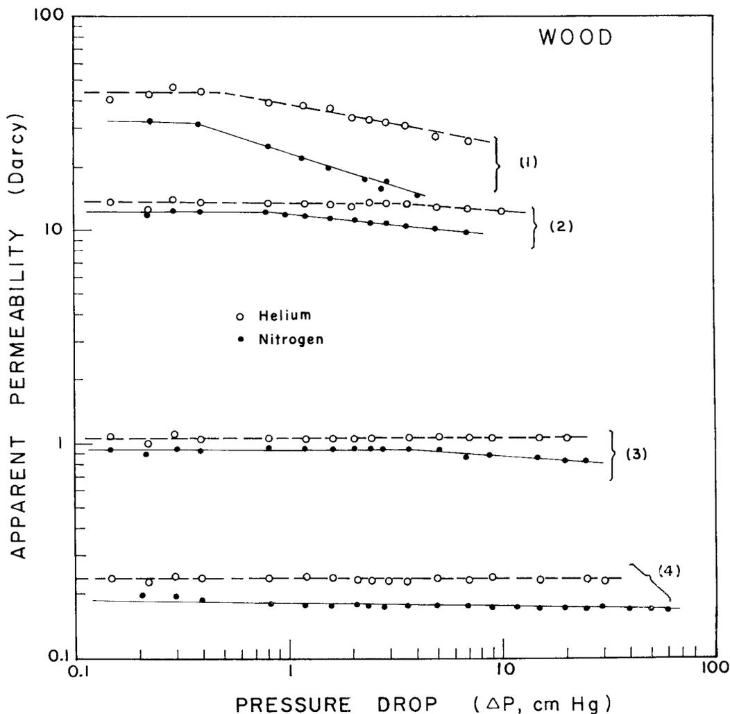
FIG. 2. Typical plot of the logarithm of apparent gas permeability as a function of the logarithm of pressure drop for several wood samples using helium and nitrogen. [(1) honeylocust, (2) soft maple, (3) hard maple, (4) hemlock.]
