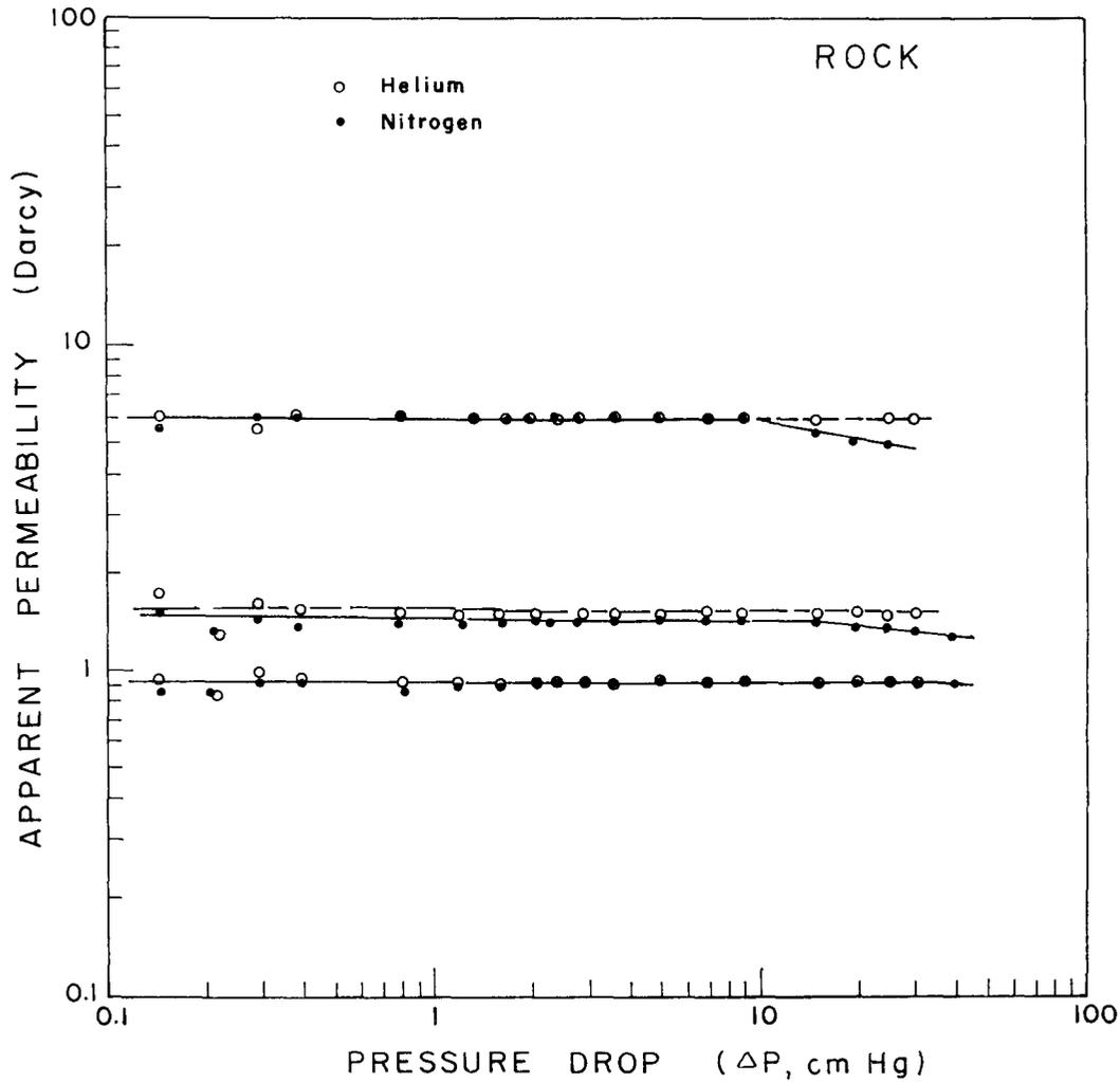
FIG. 3. Typical plot of the logarithm of apparent gas permeability as a function of the logarithm of pressure drop for three rock samples using helium and nitrogen.
