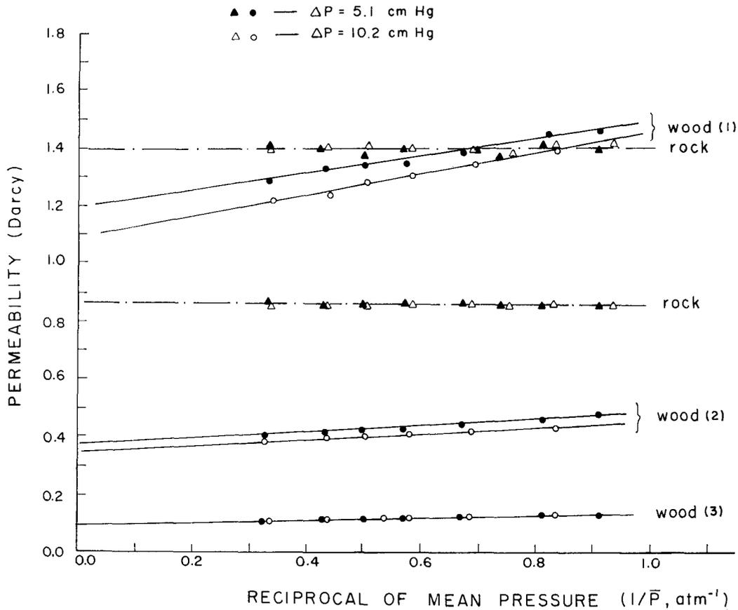
FIG. 1. Typical plot of nitrogen gas permeability as a function of reciprocal mean pressure for several wood and rock samples. [(1) white elm, (2) white pine, (3) fir.]
