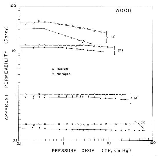
FIG. 2. Typical plot of the logarithm of apparent gas permeability as a function of the logarithm of pressure drop for several wood samples using helium and nitrogen. [(1) honeylocust, (2) soft maple, (3) hard maple, (4) hemlock.]
