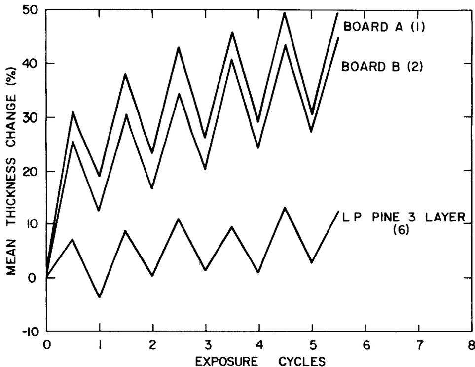
FIG. 8. Mean panel thickness change with exposure cycles for three panel types.
