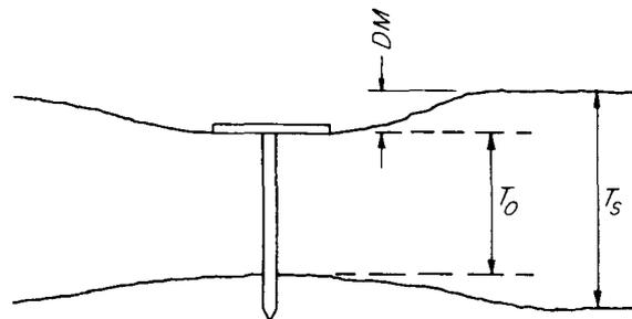
FIG. 13. Differential movement of nailhead with respect to panel thickness.
