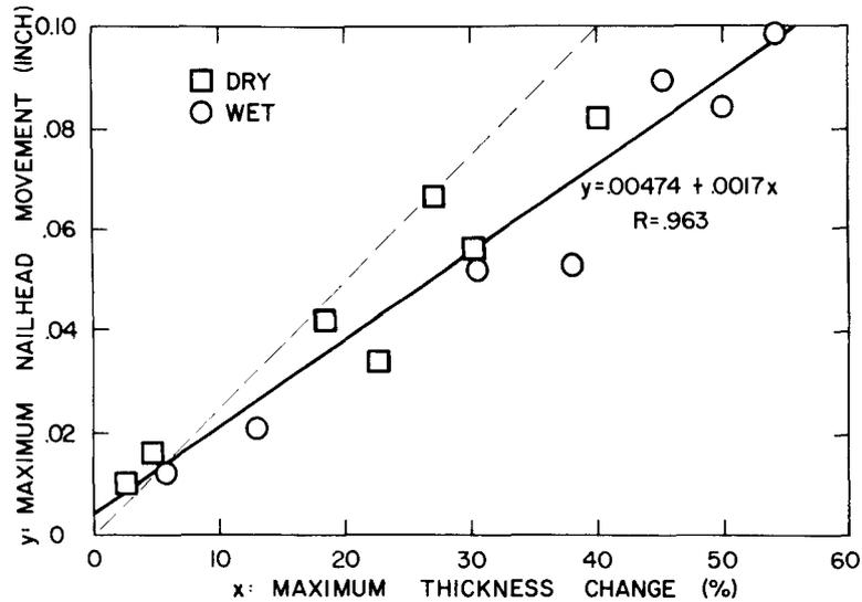
FIG. 12. Maximum recorded mean differential nailhead movements (with respect to panel surfaces) as a function of maximum mean observed panel thickness change. □: Refers to movement at end of a dry half-cycle. ○: Refers to movement at end of a wet half-cycle.
