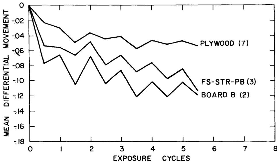
FIG. 7. Mean differential nailhead movement with respect to shingle surface for three panel types.
