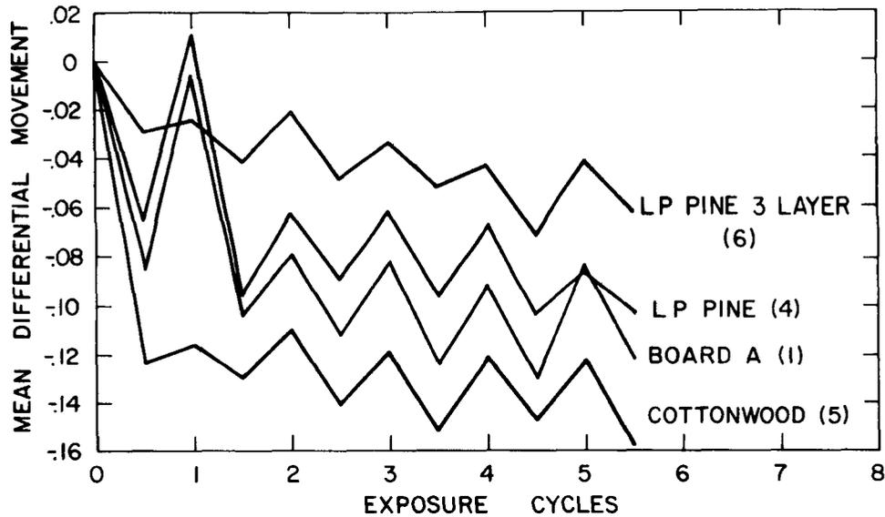
FIG. 6. Mean differential nailhead movement with respect to shingle surface for four panel types.
