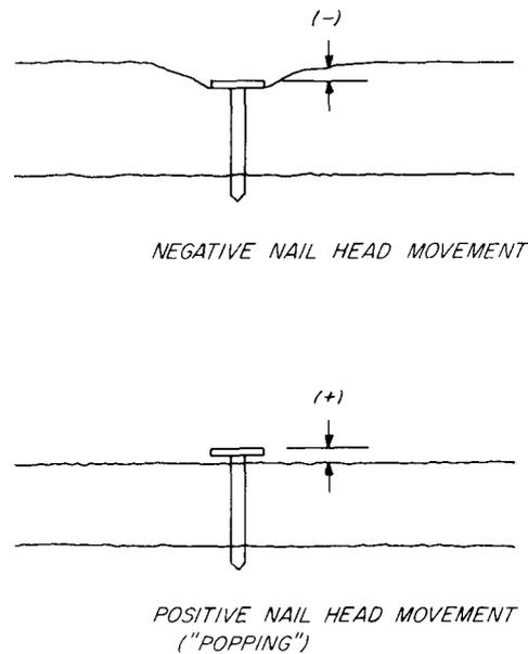
FIG. 1. Illustration of nail popping positive nail movement in panels, as contrasted with negative nail movement.
