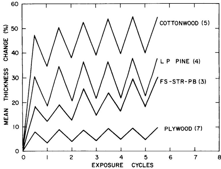
FIG. 9. Mean panel thickness change with exposure cycles for four panel types.
