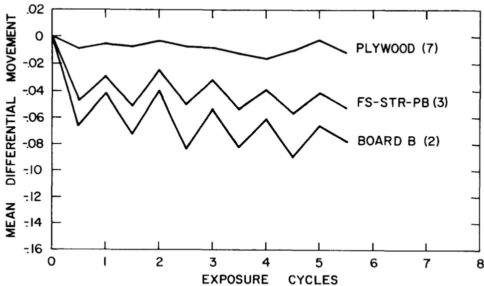
FIG. 5. Mean differential movement of nailheads with respect to panel surface for three panel types.
