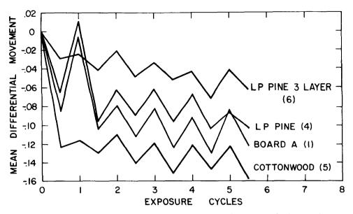
FIG. 6. Mean differential nailhead movement with respect to shingle surface for four panel types.
