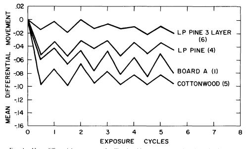
FIG. 4. Mean differential movement of nailheads with respect to panel surfaces for four panel types.
