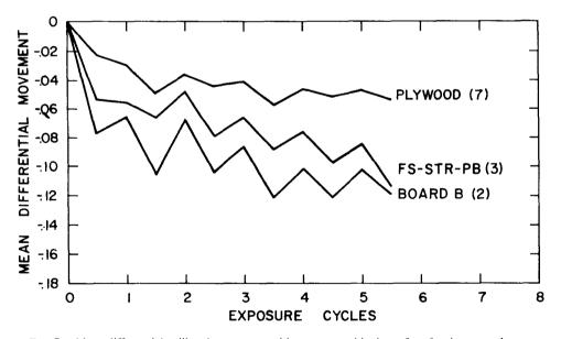
FIG. 7. Mean differential nailhead movement with respect to shingle surface for three panel types.
