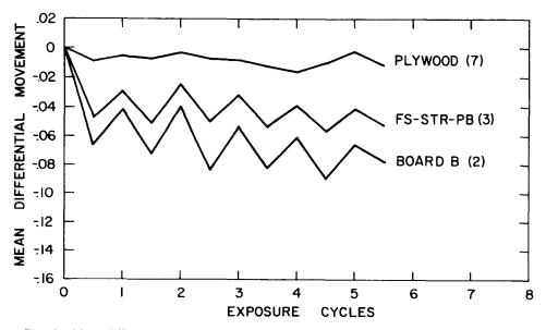
FIG. 5. Mean differential movement of nailheads with respect to panel surface for three panel types.
