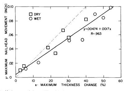
FIG. 12. Maximum recorded mean differential nailhead movements (with respect to panel surfaces) as a function of maximum mean observed panel thickness change.  $\Box$ : Refers to movement at end of a dry half-cycle.  $\odot$ : Refers to movement at end of a wet half-cycle.
