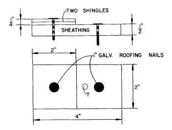
FIG. 2. Panel-shingle specimen employed in accelerated aging tests. Point "T" on specimen indicates location of thickness swell measurement.
