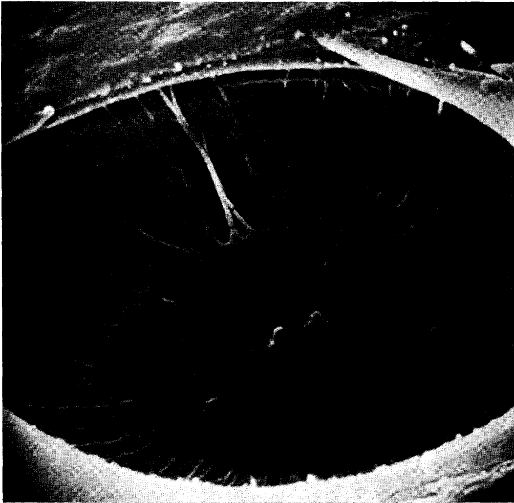
FIG. 12. A radial section viewed at a low angle and showing margo strands attached at two different rim levels. 13,400 \times
