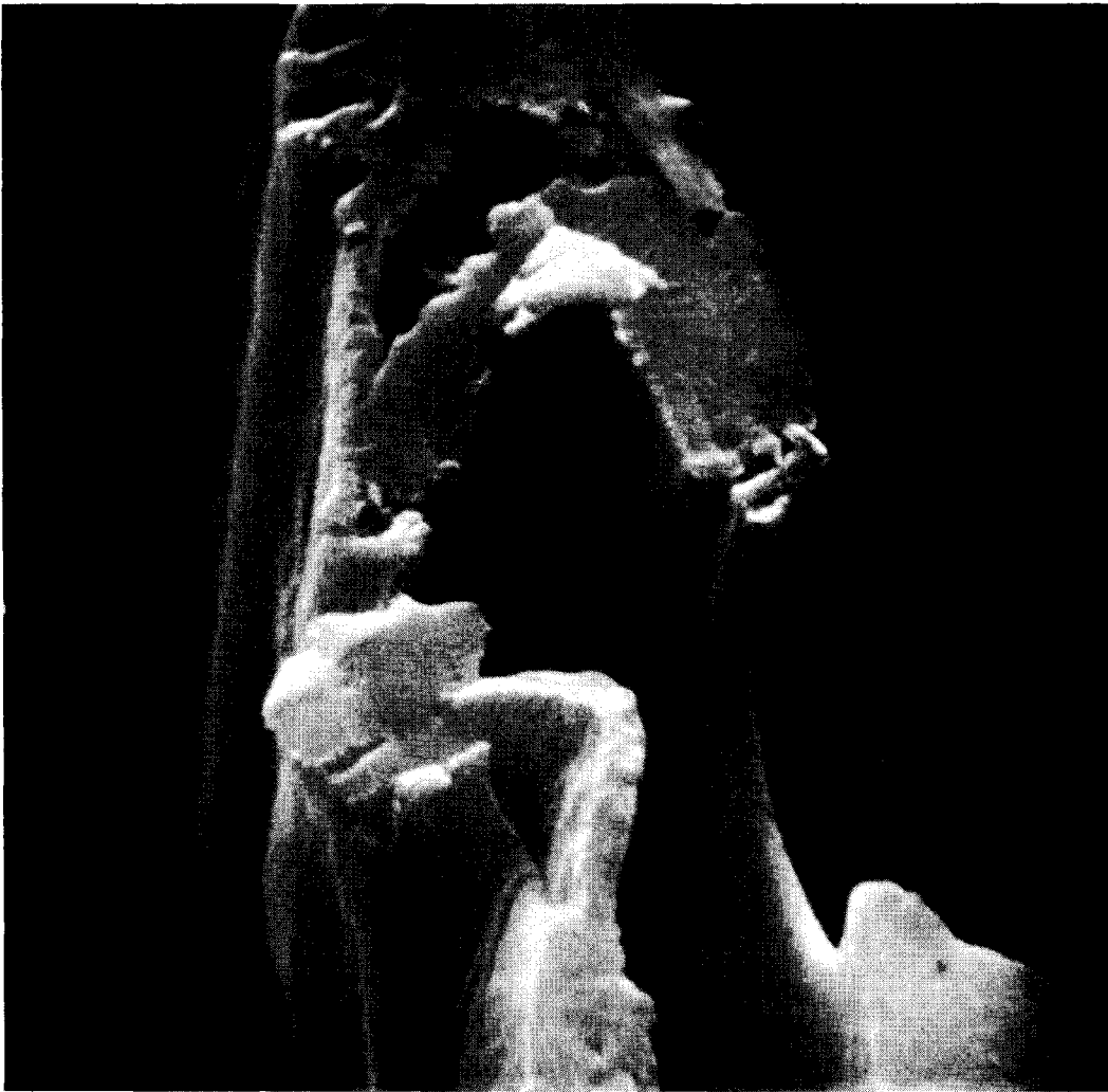
FIG. 4. A tangential view of a bordered pit aspirated to the left. The "rolled" characteristic of the aperture lip is shown. The torus was buckled by cutting action. 12,800 \times
