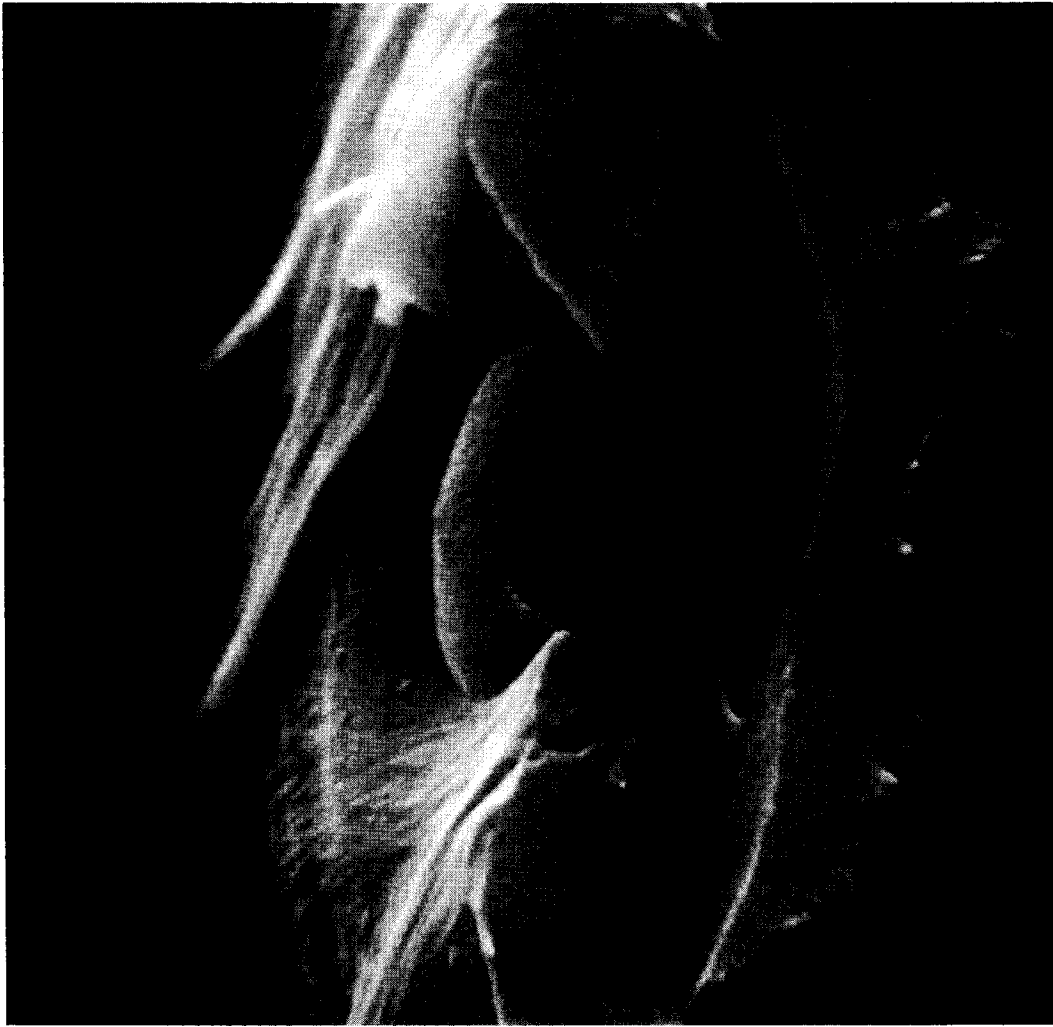
FIG. 5. A tangential view of a bordered pit aspirated to the left. The torus is very thin as compared to previous views. 12,100 \times
