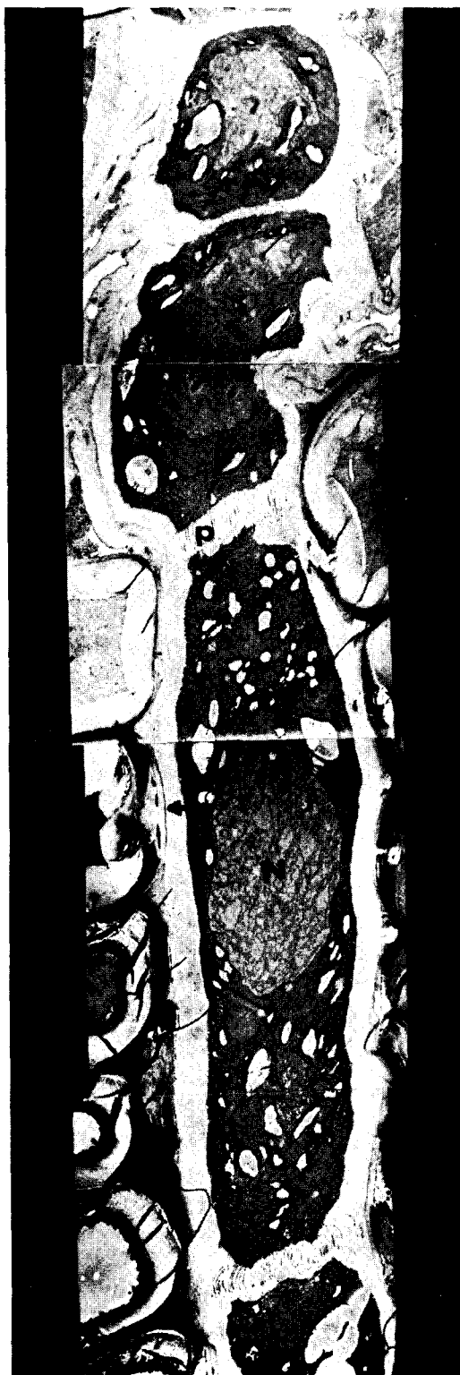
FIG. 1. Ray parenchyma cells in different stages of cell enlargement. Compare the thickness of the primary cell wall of the ray parenchyma and that of a longitudinal tracheid (arrow). Also note the large number of plasmodesmata in the tangential cell walls. Plate Nos. 6677–6680. 1900 \times .
