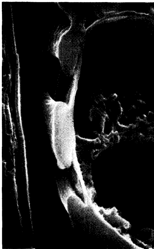
FIG. 3. Scanning electron micrograph of a ray parenchyma cell in tangential view showing the lack of secondary thickening in the ray parenchyma cell wall between pinoid pits (arrow). Cytoplasmic remains are seen inside the ray parenchyma cell. 4000 \times .
