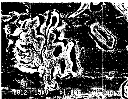
FIG. 4. Scanning electron microscope cross section of a 60% polypropylene/40% wood composite pressed to 1.0 specific gravity. Arrows point to voids between cell wall and polypropylene. Actual specific gravity is 0.695. Board was cooled after removal from press.
