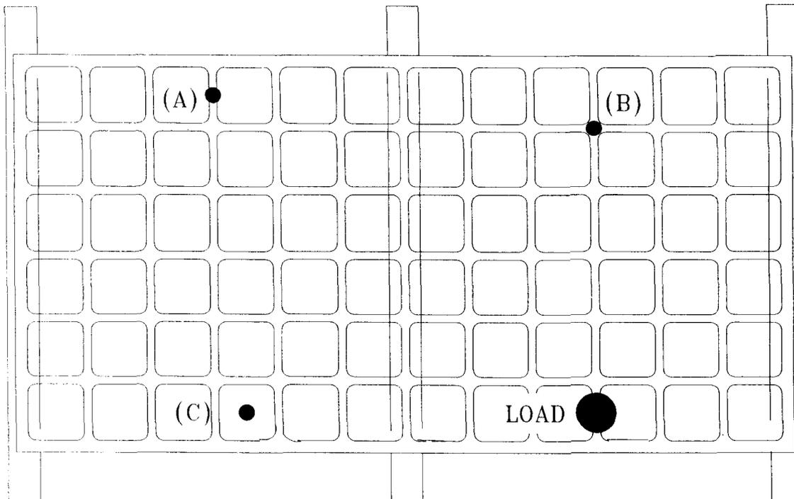
FIG. 6. 610-mm span location for static concentration load test on SBII. The large black dot indicates the position of the 76-mm loading disk. The small dots indicate puncture positions of the 25-mm disk. (A) rib, (B) rib/rib intersection, (C) face.
