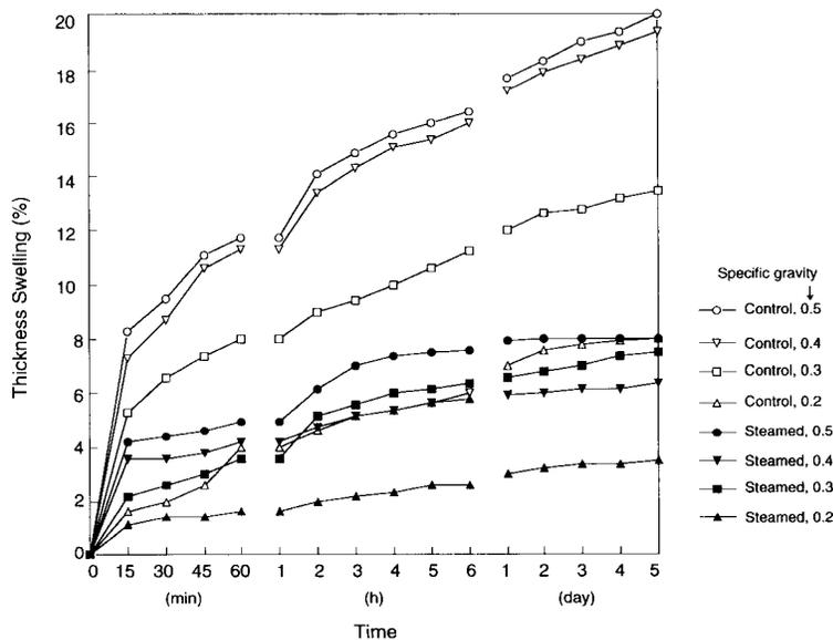
FIG. 9. Thickness swelling of untreated and steam-treated aspen fiberboards in water.
