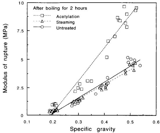
FIG. 3. Modulus of elasticity of aspen fiberboards after 2 h in boiling water.
