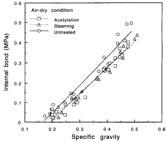
FIG. 5. Internal bond strength of aspen fiberboards at 60% RH and 20 C.
