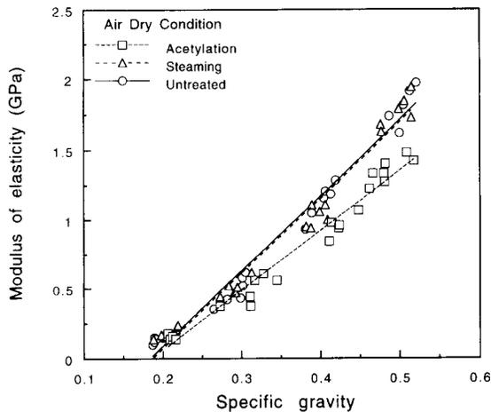
FIG. 1. Modulus of elasticity of aspen fiberboards at 60% RH and 20 C.
