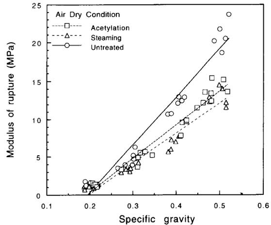
FIG. 2. Modulus of rupture of aspen fiberboards at 60% RH and 20 C.
