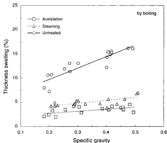
FIG. 7. Thickness swelling of aspen fiberboards after 2 h boiling.
