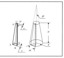
FIG. 1. A schematic diagram of a wood strip composite pole and one of its strips.
