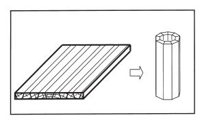
FIG. 2. A schematic diagram of a strip-cutting plan for a nine-strip composite pole.
