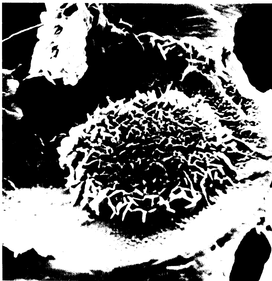
FIG. 11. Dense flaky deposits on the torus and pit annulus in wetwood, dried by ethanol solvent-exchange. SEM, 8,300 \times .
