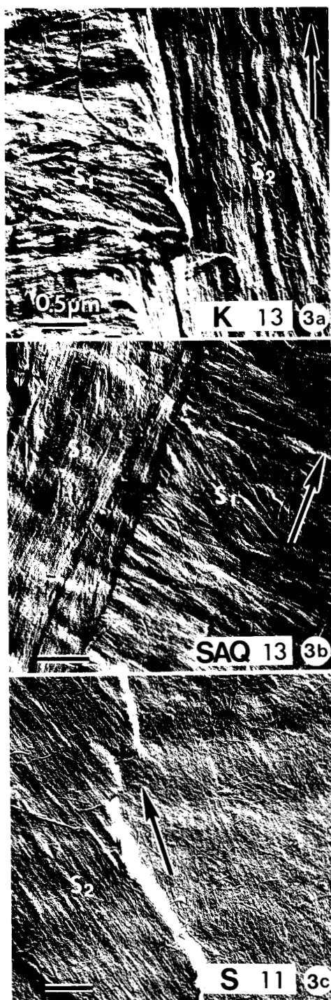
FIG. 3a–3c. Replicas of (3a) kraft (delignification = D:13%), (3b) soda/AQ (D:13%) and (3c) soda (D:11%) pulp fibers. Note that the cell-wall layers, S_1 and S_2 , are exposed. Arrows indicate the direction of the fiber axis.
